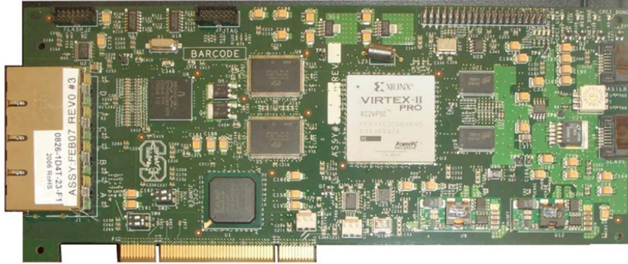
Figure B.1. The first generation NetFPGA 1G (4x1G) platform.
