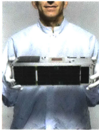
Figure 1-1: A 3U CubeSat, a common form factor used by organizations like Planet Labs, universities, and the government [1].
