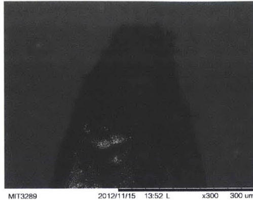
Figure 3-10: Porous nickel emitter fired in atmosphere after firing. Carbonization of the IL is evident as a result of discharges.
