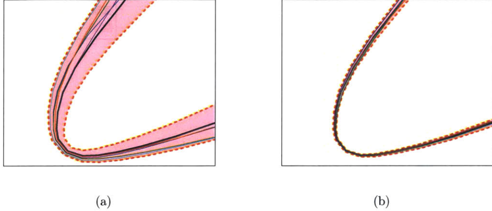
Figure 2-16: Illustration of loose (a) and strict (b) tolerances in the leading edge of a compressor blade.
