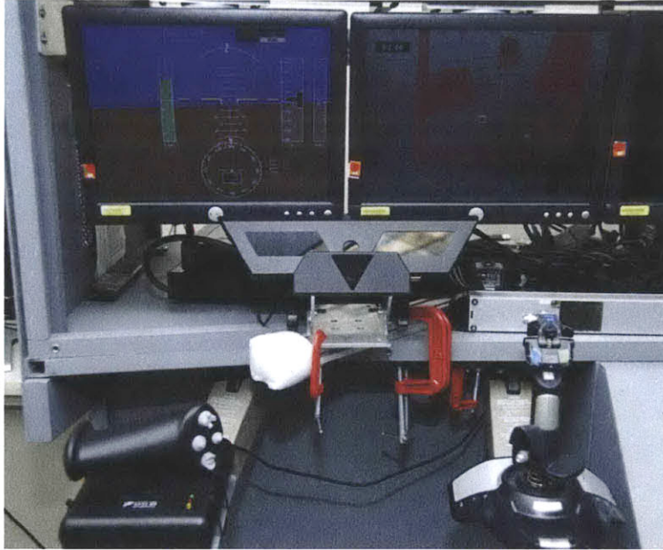
Figure 33. Location of the Tobii x50 eye tracker in the Draper Laboratory fixed-base lunar landing simulator.
