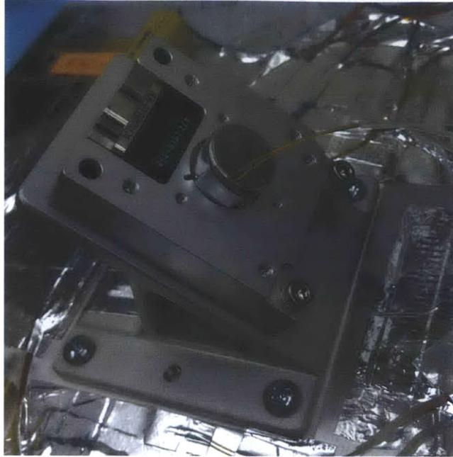
Figure A-3: SXM structure showing resistive temperature detector on SDD housing. MLI and collimator not shown.
