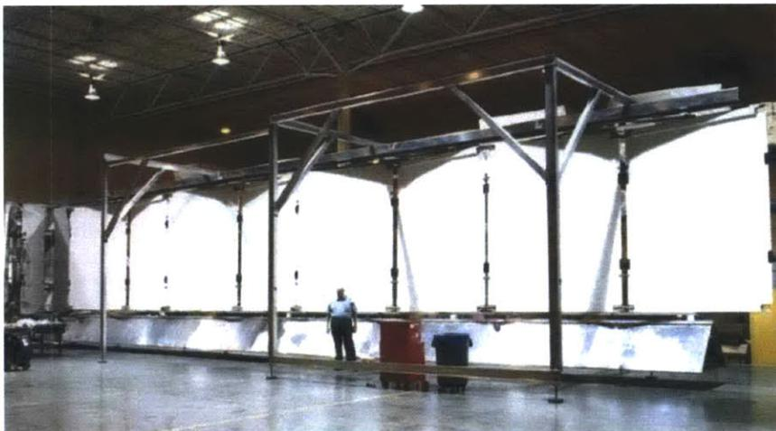
Figure 1-7: International Space Station Heat Rejection System radiator during deployment testing [40]
