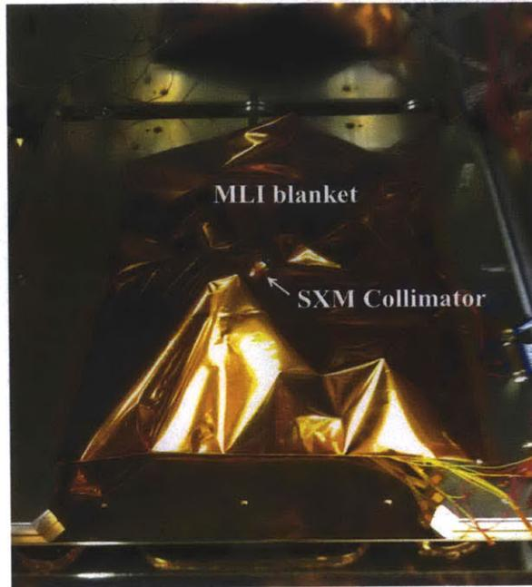
Figure A-5: Final view of SXM test article with MLI blanket in SSL thermal vacuum chamber
