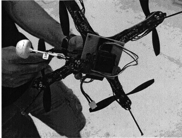
Figure 5-2: The onboard camera, wireless transmitter and antenna mounted on the quadrotor.
