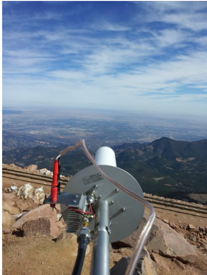
Figure 3.2: L-band helix antenna used to collect the setting occultations from the summit of Pikes Peak. The external LNA is placed directly after the antenna in the RF chain.
