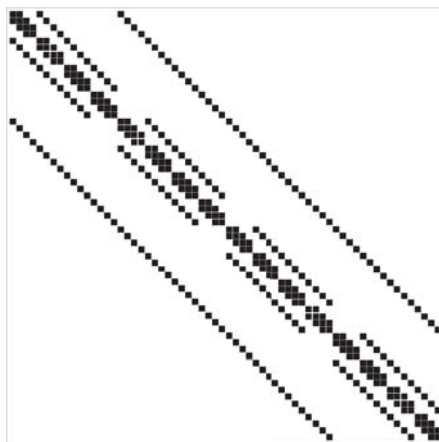
Figure 3.13: Typical implicit matrix sparsity pattern for three dimensions (up to seven unknowns per equation)
