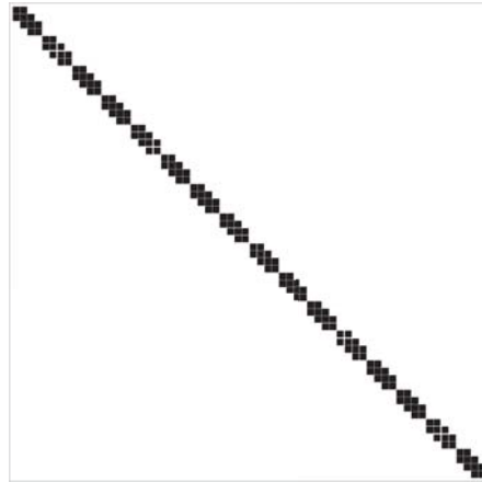
Figure 3.14: ADI matrix sparsity pattern for three dimensions (up to three unknowns per equation)
