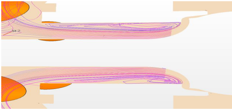
Figure 5.90. Unsteady state streamline plot at the expansion area, gap 0.002in, valve type B, time-step 0.08S.
