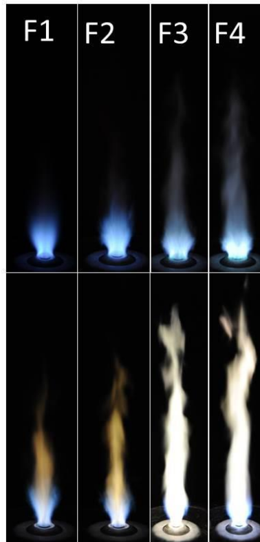
Figure 6.2: Direct flame images showing the effect of equivalence ratio at Re = 13,142 flames, top row without precursor and bottom row with precursor.
