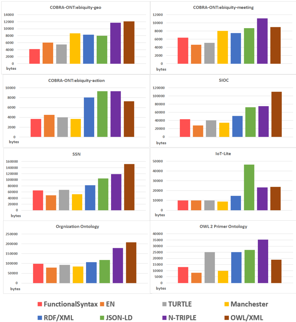
Fig. 19. Comparison of the lengths of Functional Syntax, EN and EN Schema, Turtel, Manchester Syntax, RDF/XML, JSON-LD, N-Triple, and OWL/XML with different ontologies.
