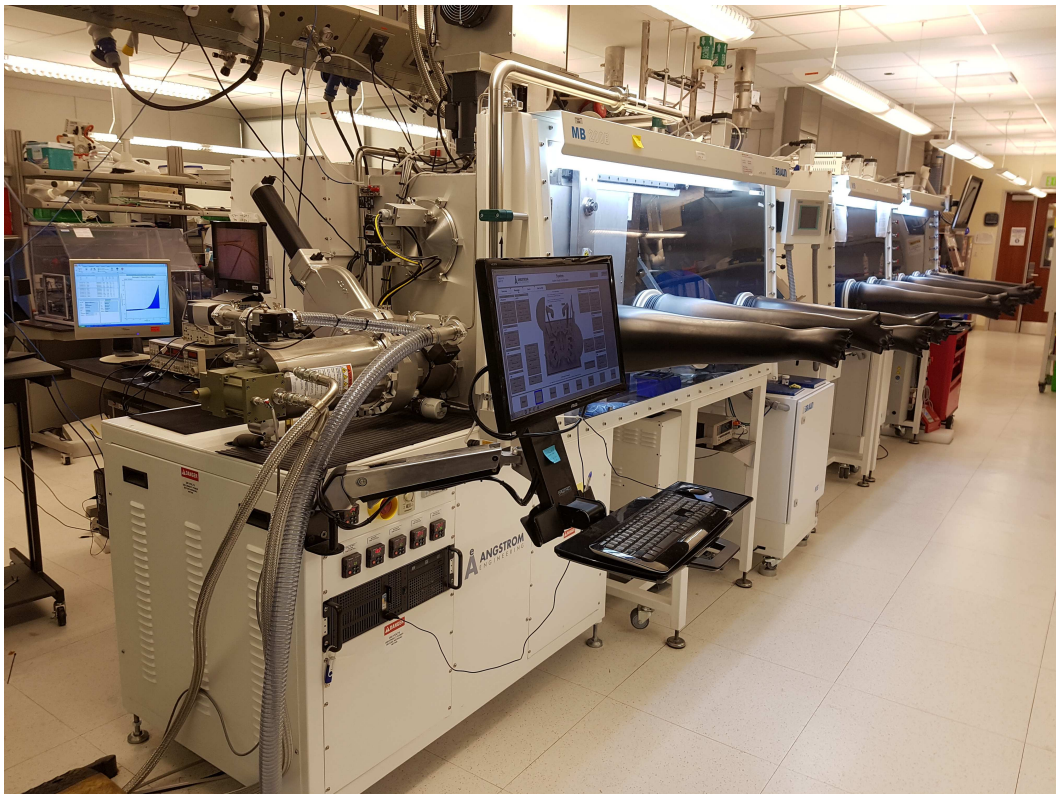
Figure 3.6: Angstrom evaporator and solar simulator housed in an Mbraun nitrogen gas filled glovebox.
