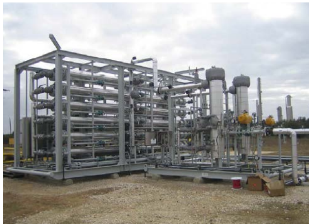
Fig. 1.8. A membrane system using commercial perfluoropolymer for CO 2 removal and hydrocarbon recovery from NG in Texas, U.S.A.
