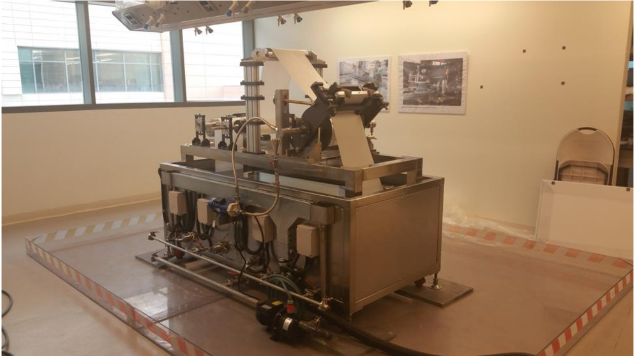
Figure 5. Flat sheet membrane machine at KAUST
