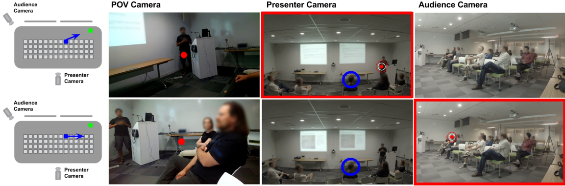
Figure 10: Egocentric FOV localization in indoor environments. The images on the first column show the room layout. The presenter is shown in Green and the person wearing Glass is shown in Blue with his egocentric view shown by the blue arrow. The second column shows the POV video frames from Glass. The red dot shows the focus-of-attention. The third and fourth column show the presenter cam and the audience cam respectively. The localization is shown by the target symbol and the selected camera is shown by the red bounding box. The person wearing Glass is highlighted by the blue circle in the presenter camera views.
