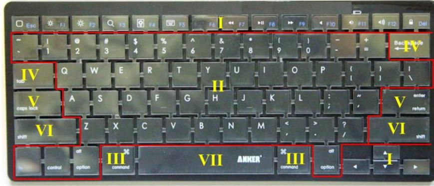
**Figure 4.8** Keys classification in the intelligent keyboard. The keys in the keyboards are classified into seven kinds according to their dimensions.<sup>112</sup>
