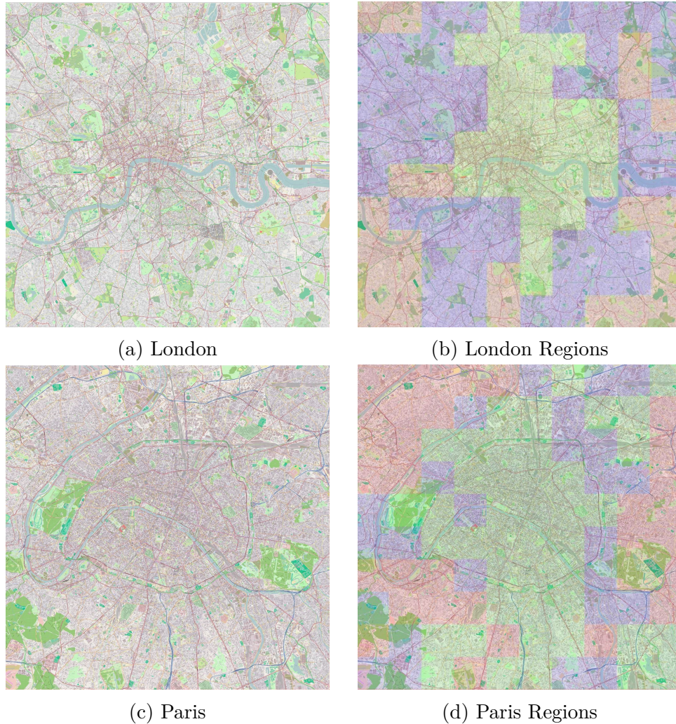
Figure 5.7: Using K-Means clustering [12] to identify city levels for London and Paris (left) into three regions (right) which are downtown (green), mid-zone (blue), and outskirts (red).
