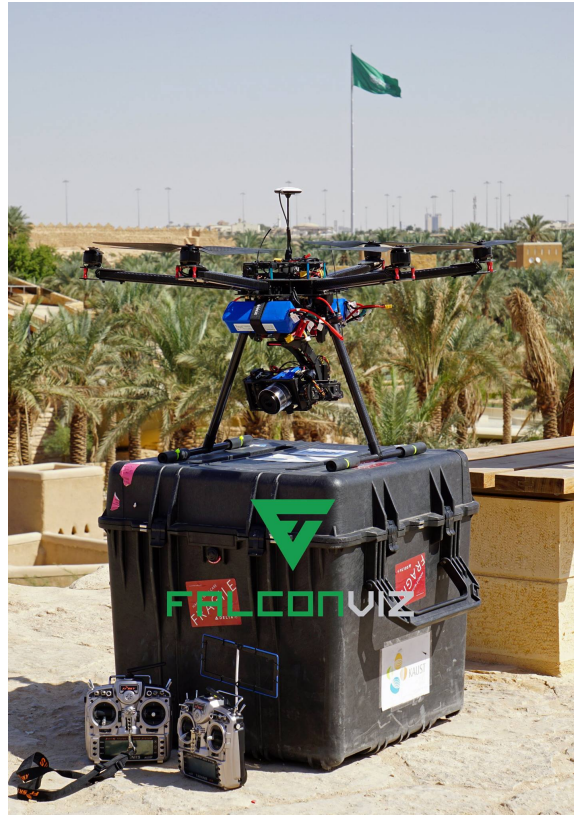
Figure 1.4: FalconViz hexacopter for 3D aerial scanning and modeling. Figure courtesy [3].
