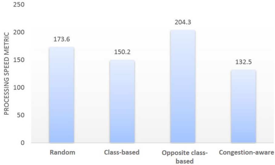
Figure 4.5: An evaluation of the processing speed metric for different storage assignment policies. The proposed optimal assignment has the fastest processing speed value (around 20-25% improvement).
