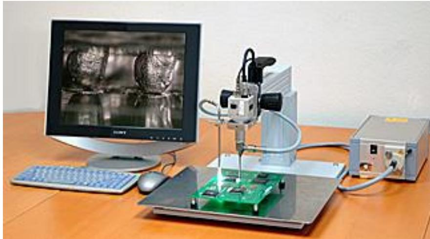
Figure 1-3: Solder balls inspection using an endoscope (Courtesy of Caltex Scientific)
