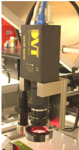
Figure 3-9: DVT series 600 smart sensor for fiducial mark locating
