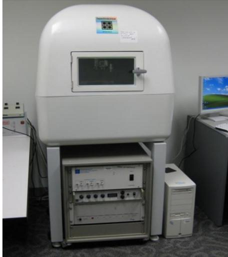
Figure 6-49: Nanoindentation tool from Hysitron
