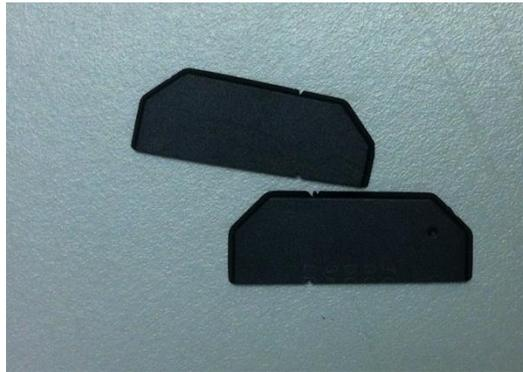
Figure 6-48: Molding compound sample for nanoindentation
