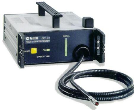
Figure 3-6: Polytec OFV-511 heterodyne interferometer (Source: Polytec®)
