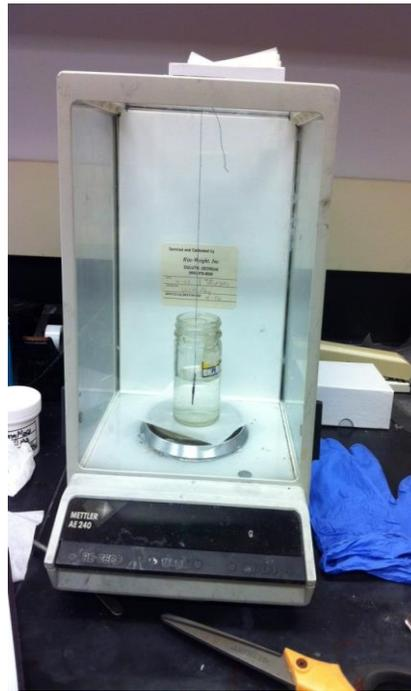
Figure 6-52: Experimental setup for density measurement
