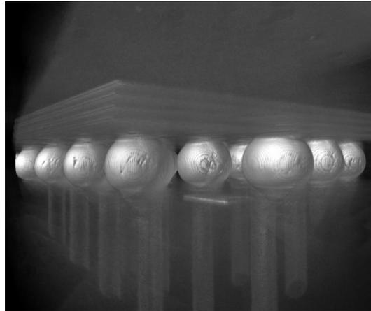
Figure 6-11: 3D X-ray Images for solder ball A1 on Chip6 and its neighboring solder balls
