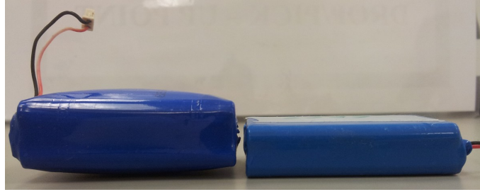
Figure 2.6: Left: effects of high outdoor temperature and high charge on a Li-ion battery. Right: A new Li-ion battery
