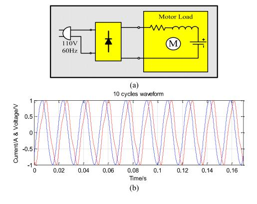
Figure 3.4 (a) The conceptual front-end circuit of inductive loads; (b) Normalized steady state voltage and current waveform of inductive loads.
