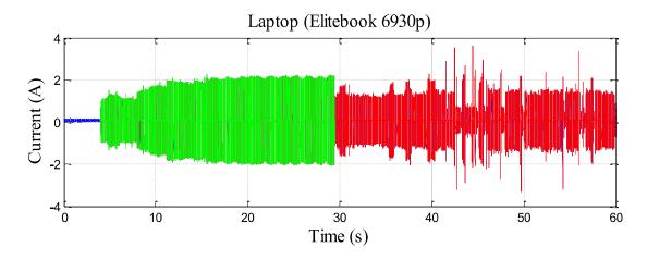
Figure 3.16 The start-up current of a typical laptop.
