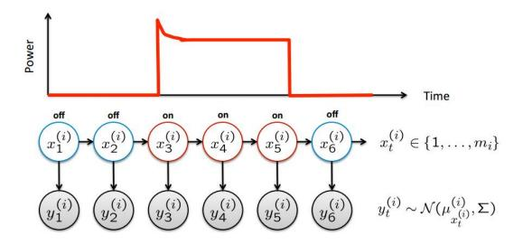
Figure 2.11 HMM model of the kitchen outlets [83].
