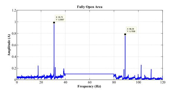
Figure 6.18 The eccentricity harmonics of AHU under the fully open area scenario.
