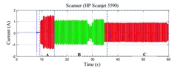
Figure 3.18 The start-up current of a typical scanner.
