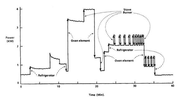
Figure 2.6 Power vs. time plot shows step changes due to individual appliance events [20].
