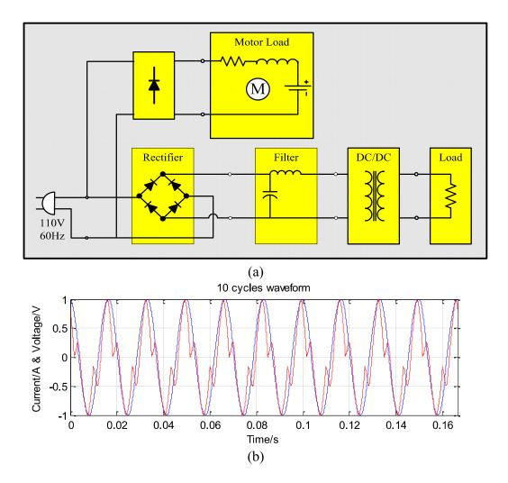
Figure 3.13 (a) The conceptual front-end circuit of complex structure load; (b) Normalized steady state voltage and current waveform of complex structure load.
