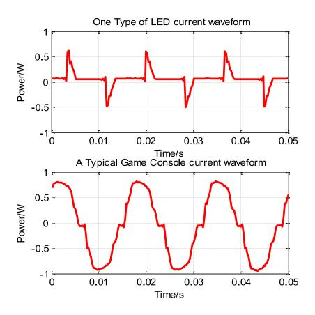
Figure 4.3 The current waveforms of a LED bulb and a game console.
