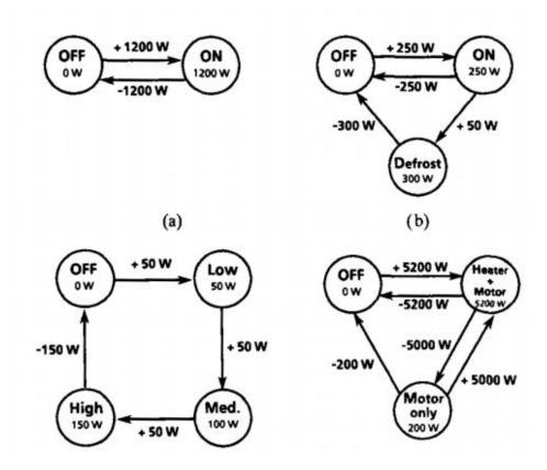
Figure 2.8 Finite-state appliance models: (a) generic 1200 W two-state appliance, e.g., toaster; (b) refrigerator with defrost state; (c) "three-way" lamp; (d) clothes dryer [109].
