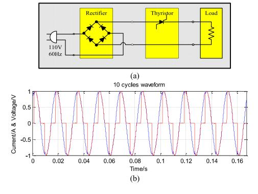
Figure 3.12 (a) The conceptual front-end circuit of PAC controllable load; (b) Normalized steady state voltage and current waveform of PAC controllable load.
