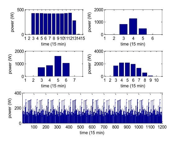
Figure 5.12 Individual load waveforms in the aggregated signal. From top to bottom, left to right: APP1, APP2, APP3, APP4 and brown loads.
