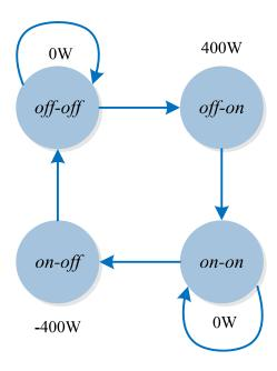
Figure 5.2 A typical state transition diagram of HMM aiming at modeling first-order power difference of loads.
