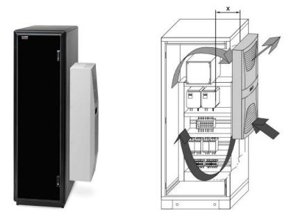
Figure 6.24 The concept figure of an enclosure air conditioner.
