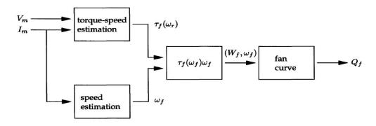
Figure 2.12 Flowchat of the air-flow estimation method [128].
