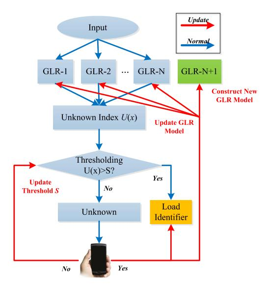
Figure 4.6 The flowchart of the proposed unknown model detection algorithm.
