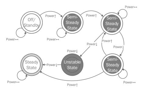
Figure 3.26 The finite state machine model of a scanner.
