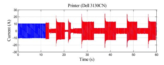
Figure 3.20 The working current of a typical printer.
