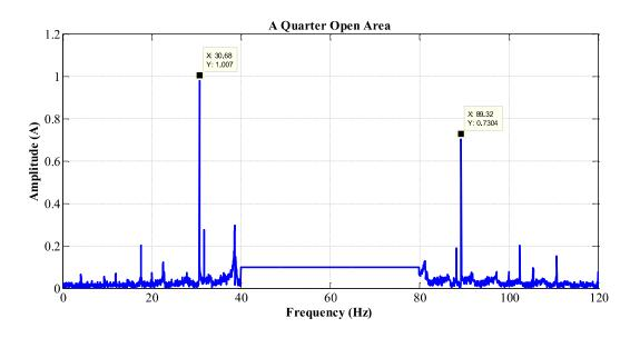
Figure 6.20 The eccentricity harmonics of AHU under the a quarter open area scenario.
