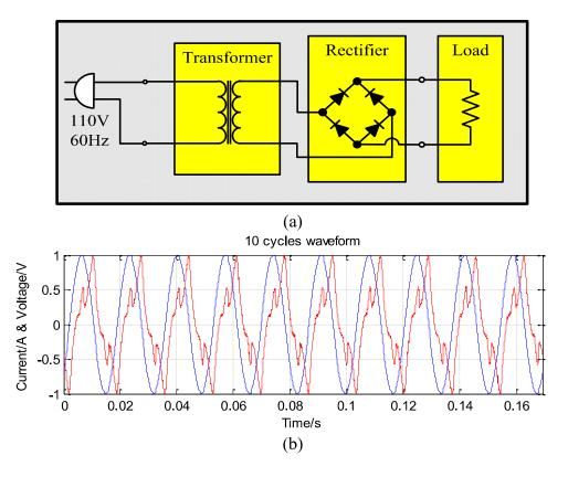
Figure 3.11 (a) The conceptual front-end circuit of linear power supply; (b) Normalized steady state voltage and current waveform of linear power supply.
