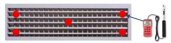
Figure 6.15 Airflow speed measurement points.
