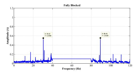
Figure 6.22 The eccentricity harmonics of AHU under the fully blocked scenario.
