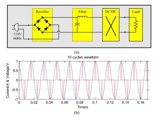
Figure 3.5 (a) The conceptual front-end circuit of ELw/oP; (b) Normalized steady state voltage and current waveform of ELw/oP.
