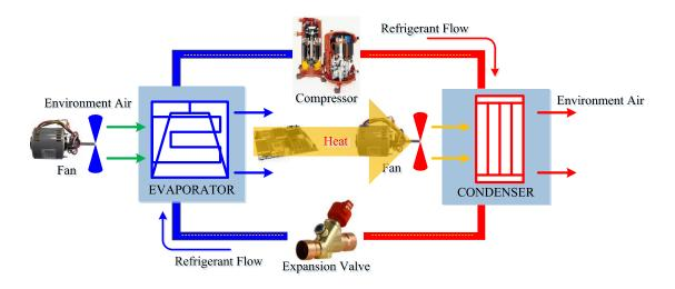
Figure 6.25 Air conditioning cycle schematic diagram.
