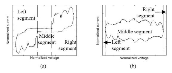
Figure 2.5 (a) The trajectories of a laptop, (b) a desktop PC operating in standby mode [105].
