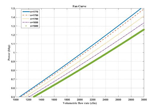
Figure 6.9 Fan curves of the AHU based on (6.13).
