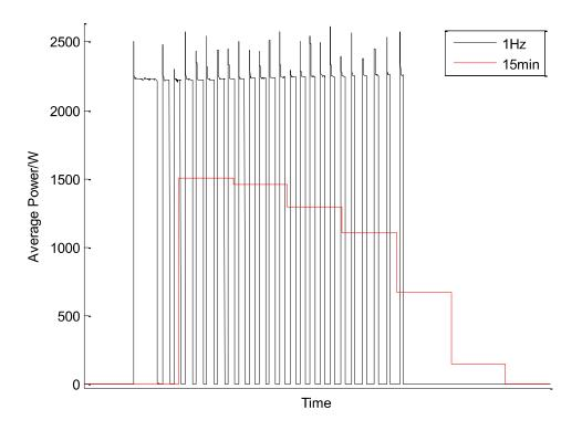
Figure 1.5 The difference between 1Hz and 15 minutes resolution data.
