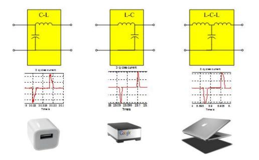
Figure 3.7 Three kinds of filters in power supply and their representative load types e.g. a cellphone charger, a set top box, and a laptop.
