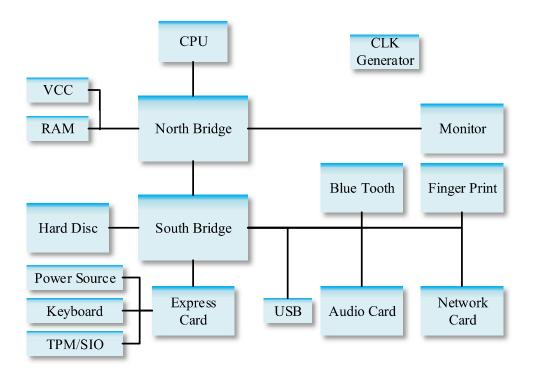
Figure 3.15 The structure of a typical laptop.
