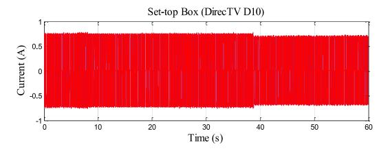
Figure 3.19 The start-up current of a typical set-top Box.
