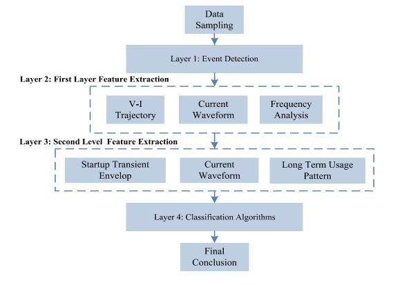
Figure 3.2 A hierarchical structure of NILM system.
