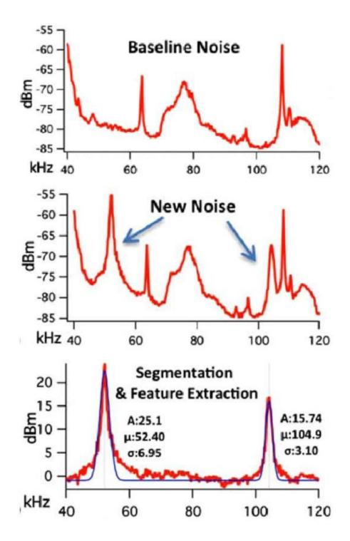
Figure 2.3 Background noise observed in a socket (upper panel). A new SMPS device is turned on, producing additive EMI (middle panel). After background subtraction the new signal features are extracted. The features are amplitude (A), mean ( $\mu$ ) and variance ( $\sigma$ ) of the Gaussian fit [103].
