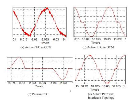
Figure 3.10 Different waveforms in terms of different PFC modules.
