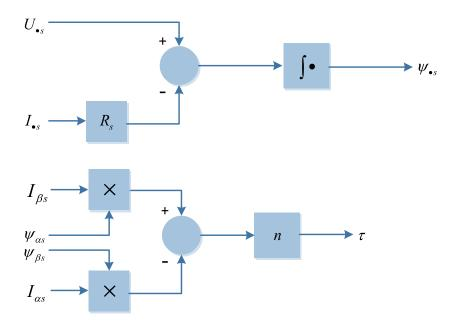
Figure 6.4 Dynamic torque estimation model.
