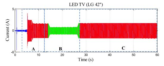
Figure 3.21 The start-up current of LCD/LED TV.
