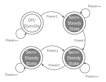
Figure 3.25 The finite state machine model of a scanner.
