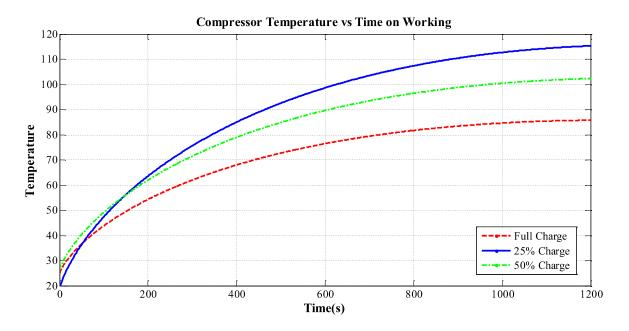
Figure 6.32 Estimated temperature curves of the three studied refrigerant conditions.
