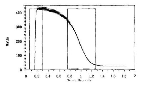
Figure 2.9 Measure induction motor real power transient [100].
