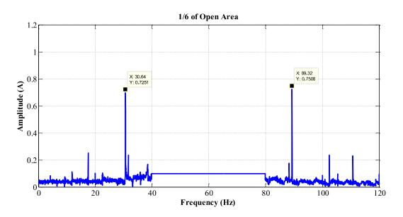
Figure 6.21 The eccentricity harmonics of AHU under the 1/6 of open area scenario.
