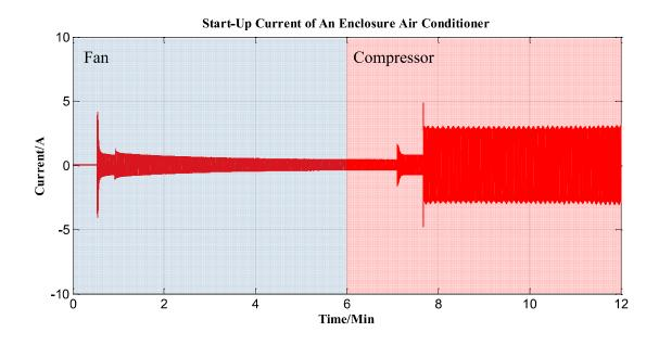
Figure 6.29 Start-up current of an enclosure air conditioner.
