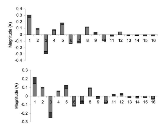
Figure 2.2 Harmonic signatures of monitor (upper) and CPU (lower). The fluctuations are shown by black bars [97].
