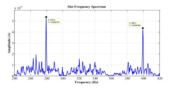
Figure 6.30 A sample slip frequency spectrum of the studied air conditioner.
