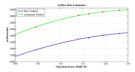
Figure 6.23 Regression analysis for airflow against the vibration power of AHU.
