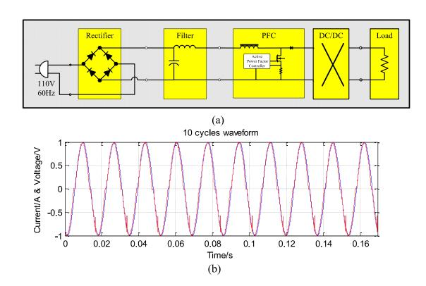
Figure 3.8 (a) The conceptual front-end circuit of P-Category; (b) Normalized steady state voltage and current waveform of ELwP.
