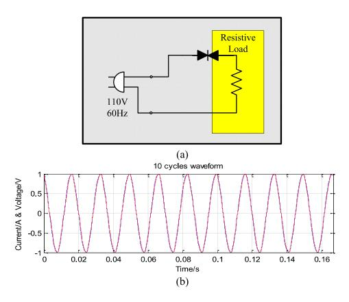
Figure 3.3 (a) The conceptual front-end circuit of pure resistive loads; (b) Normalized steady state voltage and current waveform of pure resistive loads.
