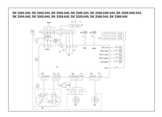
Figure 6.28 Electric circuit scheme of the air conditioner.
