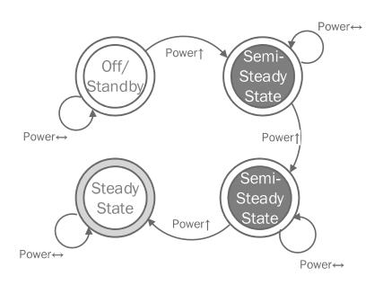
Figure 3.24 The finite state machine model of a monitor.
