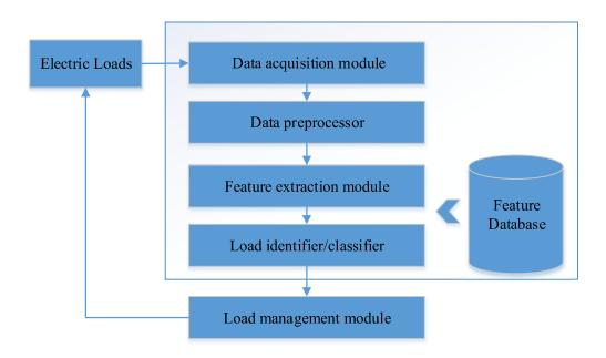
Figure 1.2 System structure for the non-intrusive load monitoring technology.
