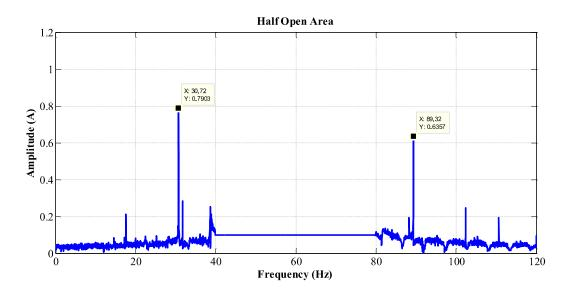
Figure 6.19 The eccentricity harmonics of AHU under the half open area scenario.
