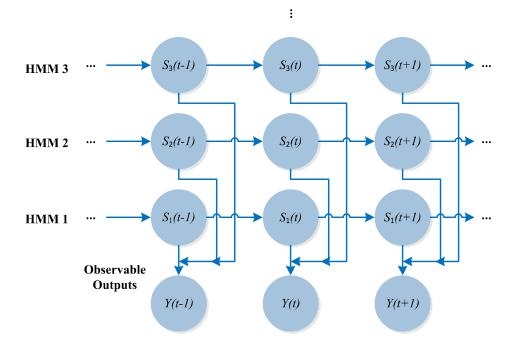
Figure 5.1 Architecture of factorial-HMM.
