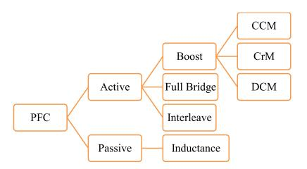
Figure 3.9 A classification of PFCs with different structures and different control strategies.
