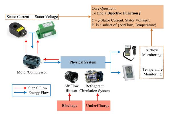
Figure 6.1 Architecture of electrical measurement based fault detection of HVAC.
