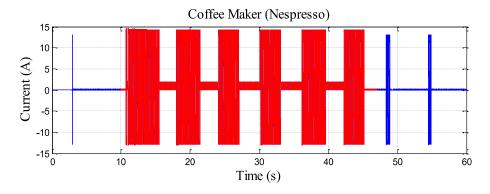
Figure 3.14 The working current of a typical coffee maker.
