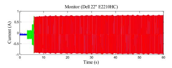
Figure 3.17 The start-up current of a typical monitor.
