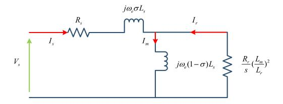
Figure 6.5 The steady-state equivalent circuit of an induction machine.
