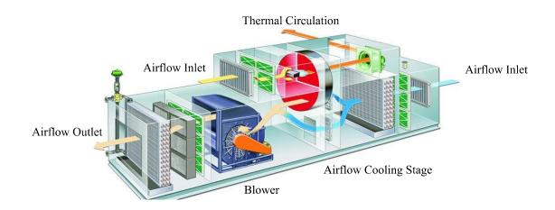
Figure 6.6 A typical AHU scheme.
