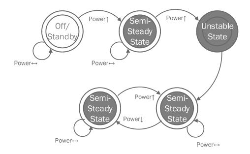
Figure 3.23 The finite state machine model of a laptop.
