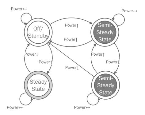
Figure 3.22 The finite state machine model of a coffee maker.
