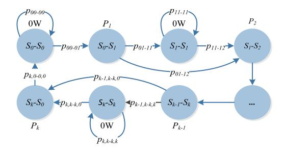
Figure 5.9 State transition diagram of HMM with predefined initial parameters.
