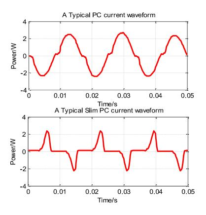
Figure 4.2 Two typical PC current waveforms.
