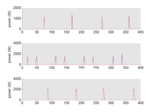
Figure 5.13 Disaggregated power signal in the first iteration. Blue line denotes the disaggregated power signal; red line denotes true measured circuit-level power signal.
