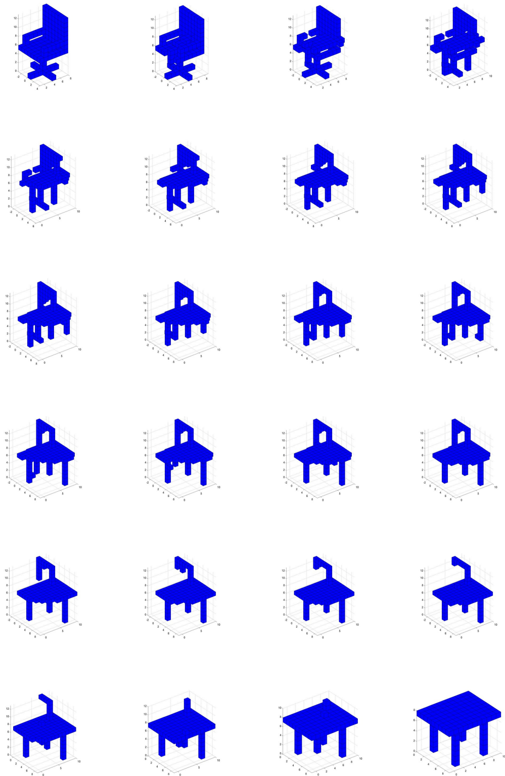
Figure 14: Example of a homogeneous reconfiguration sequence showing a reconfiguration from a chair to a table configuration.
