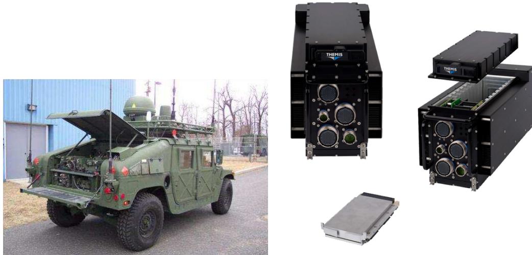
(a) HPC mounted on a military vehicle. (b) A sample HPC module, TSY-300X 3U VPX by Themis Computers [20].
