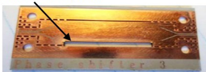
Fig. 2.7. Ferrite loaded SIW based phase shifter using external magnets [44]
