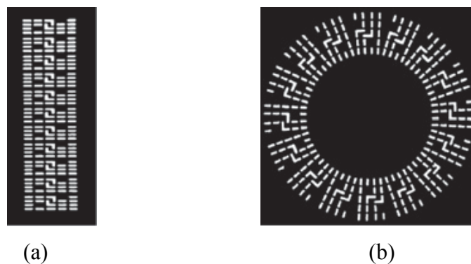
Fig. 2.13. Embedded bias windings (a) solenoid (b) toroid [62], [63]
