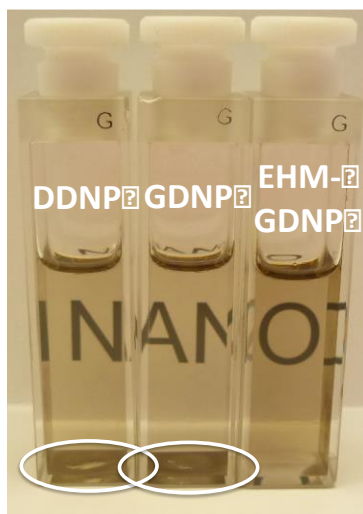
Figure 4.5 Dilute solutions of DDNPs (left), GDNPs(800) (center) and EHM-treated GDNPs(800) (right) in chlorobenzene (same initial concentration). After 3 days, the colloidal solution of EHM-GDNPs remains stable, while the unfunctionalized DDNP and GDNP precursors precipitated and settled at the bottom of the quartz cuvettes (white circled).
