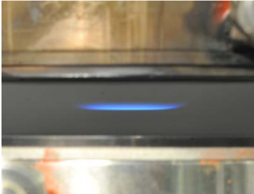
Figure 1.6 Typical nonpremixed counterflow flame.
