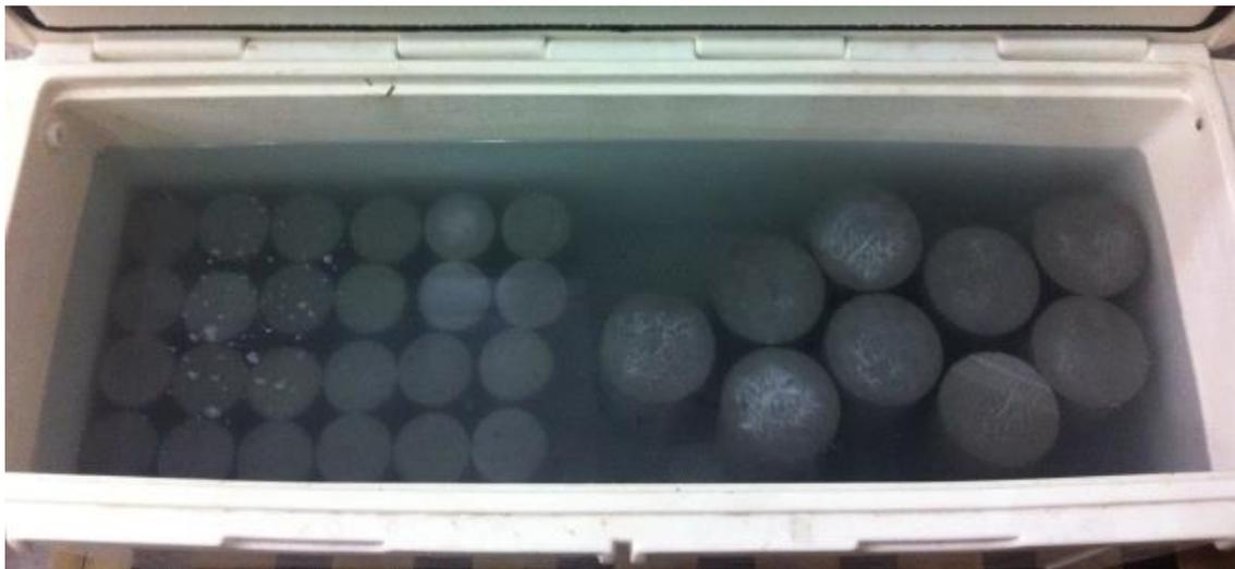
Figure 3.17: Specimens in match-curing storage tank
