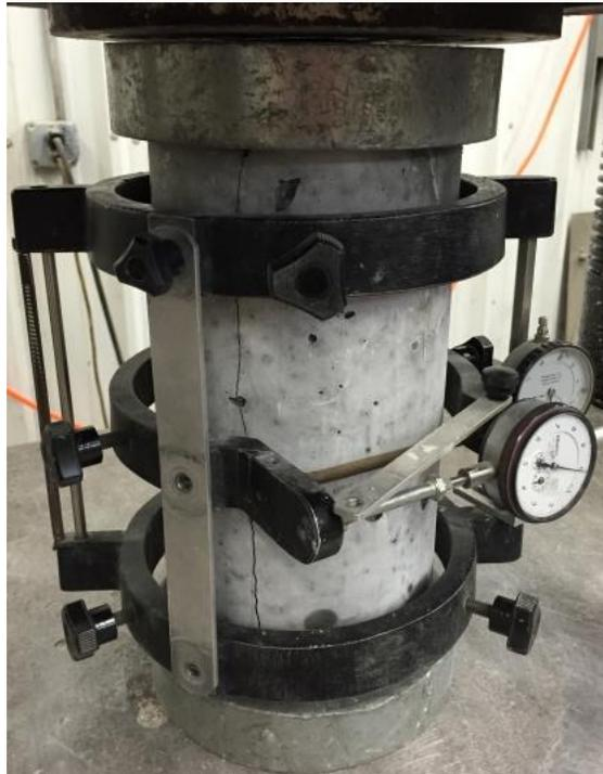
Figure 3.30: Cracked specimen from modulus of elasticity and Poisson's ratio testing
