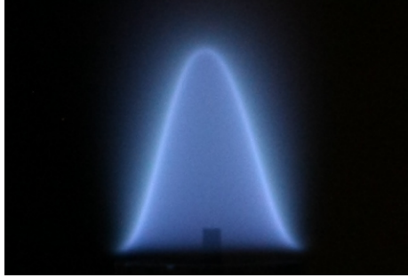
Figure 2.7: Bunsen-type stoichiometric methane/air premixed conical flame. Image courtesy of Dr. Deanna Lacoste.
