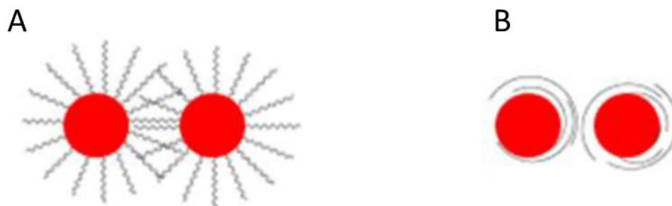
Figure 1.7 Steric stabilization of NPs; a) short and b) long surfactant chains.
