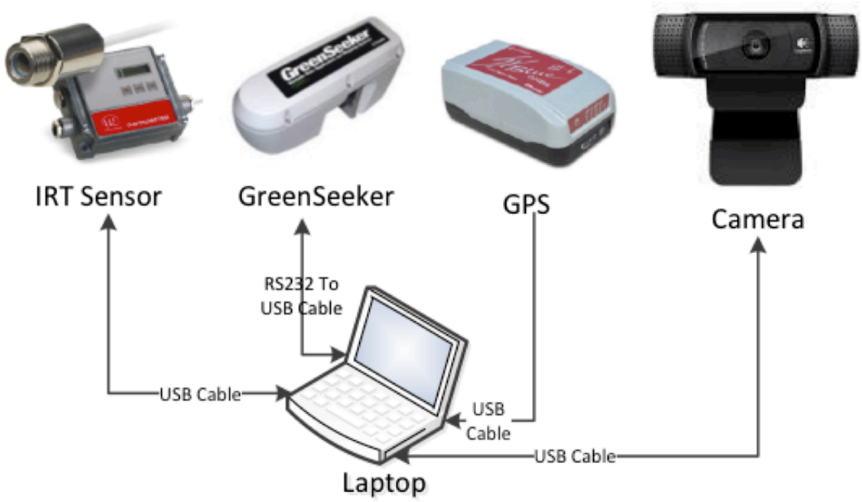
Figure 2-1. Integrated hardware components of Phenocart.
