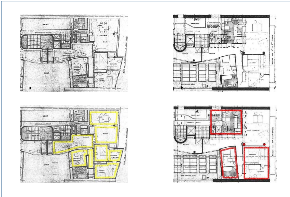
Figure 6.2: The old (upper left) and new (upper right) plans for the apartment building, with spatial blocks outlined (lower row) (Source: Bafna, 2004)
