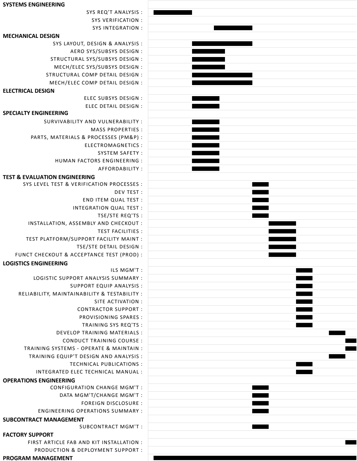
Figure 53: Gantt Chart Depicting P-BEAT Development Process Order and Dependencies with Notional Task Durations
