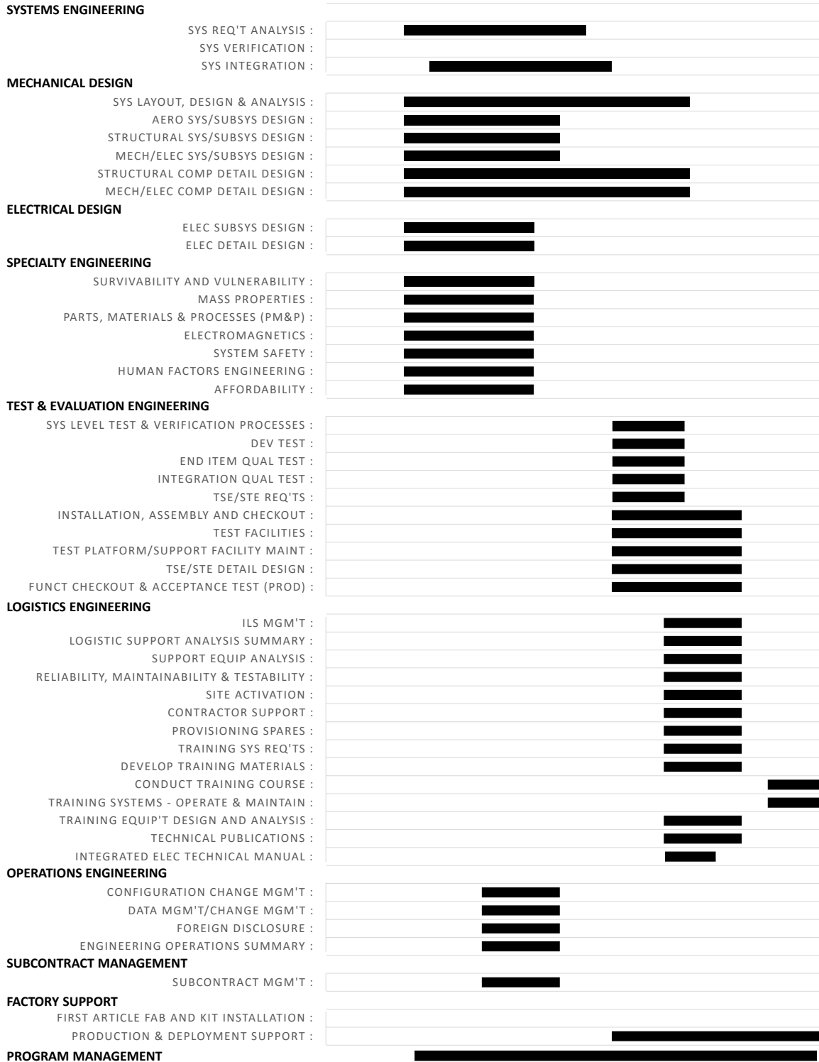
Figure 106: Gantt Chart Depicting Optimistic (Parallel) P-BEAT Development Process Order and Dependencies with Notional Task Durations
