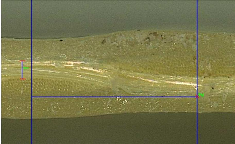
Figure C.2: Kevlar<sup>®</sup> 49 Cross-Section Image Taken Using Keyence Digital Microscope with 150 X Magnification
