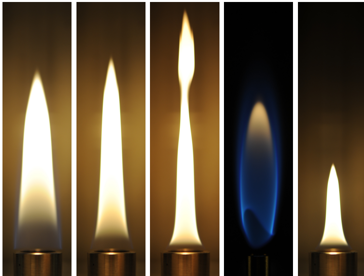
Figure 4.2: From (l) to (r): stable, transition, flickering, lifted, and wavy flames.
