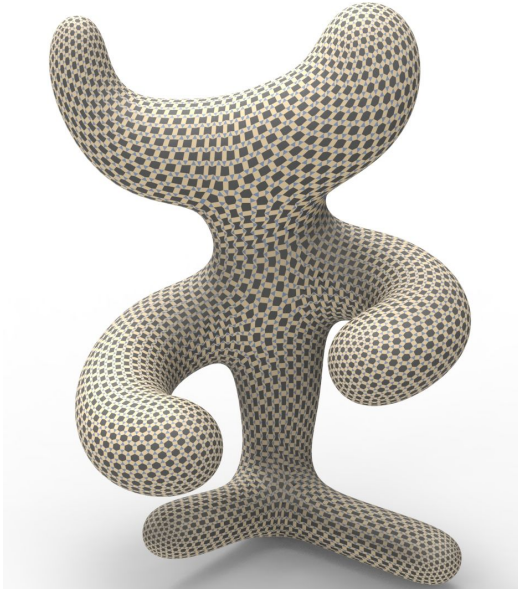
Figure 4.18: We show a (3, 4, 6, 4) pattern on the Moomoo model with 57 singularities. This is the most complicated model shown in the chapter due to the high number of singularities (hexagons replaced by septagons and pentagons) and the high curvature variations.
