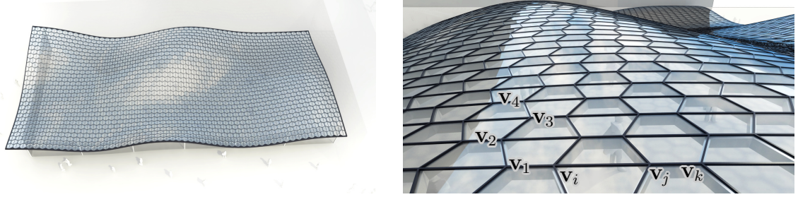
Figure 3.10: Zigzag quadrangulation: We show two views of a polyhedral quad mesh equipped with a honeycomb support structure, approximating the design surface of the Cour Visconti roof in the Louvre, Paris (see also Figure 1.2). The right hand image illustrates the “zigzag” mesh polylines (with consecutive vertices \mathbf{v}_1, \dots, \mathbf{v}_4 ) and “straight” mesh polylines (with consecutive vertices \mathbf{v}_i, \mathbf{v}_j, \mathbf{v}_k ). Fairness of these polylines is a topic of optimization.
