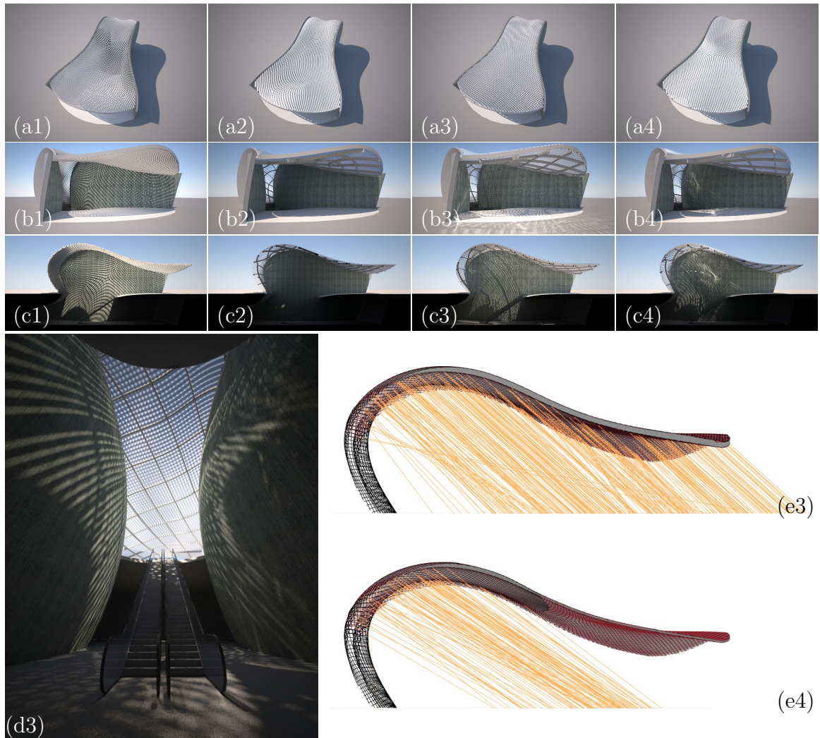
Figure 2.10: Shading and lighting systems for a subway entrance in London at noon, June 21. Rows a–d represent top view, front view, cross-section, and interior view, respectively. Columns 1–4 correspond to different shading systems extracted from a congruence \mathcal{L} : In (a1)–(c1) \mathcal{L} consists of the normals of the mesh A which represents the roof, so the support structure follows the principal curvature lines of A . There is no effective shading. In (a2)–(c2) \mathcal{L} is optimized for blocking sunlight. In (a3)–(e3) \mathcal{L} is optimized such that shading fins reflect sunlight towards the interior at an angle of 45 degrees, with (e3) illustrating reflected light rays. In (a4)–(e4) the front part of the roof is optimized for shading, the rest for reflection.
