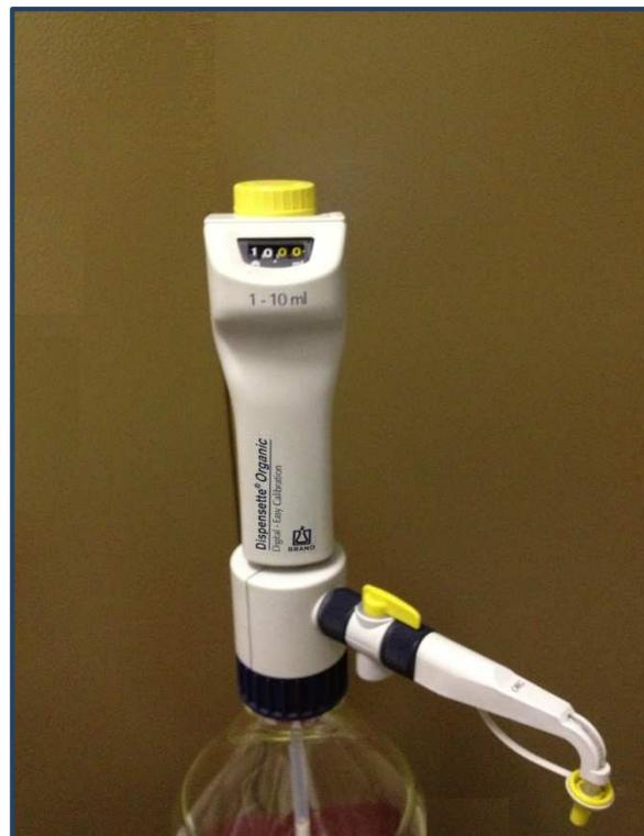
Figure 4: Dispensette Organic dispenser with a readability of 0.01 ml and an accuracy of 0.005 ml
