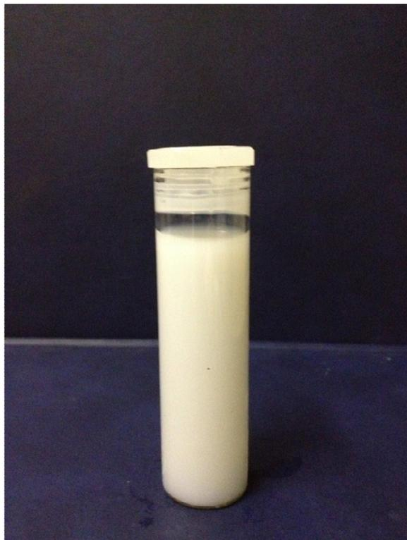
**Figure 8: SiO<sub>2</sub>-water 4% nanofluid**
