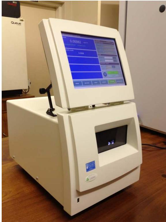
**Figure 9: Rudolph Research Analytical DDM 2911 digital density meter**
