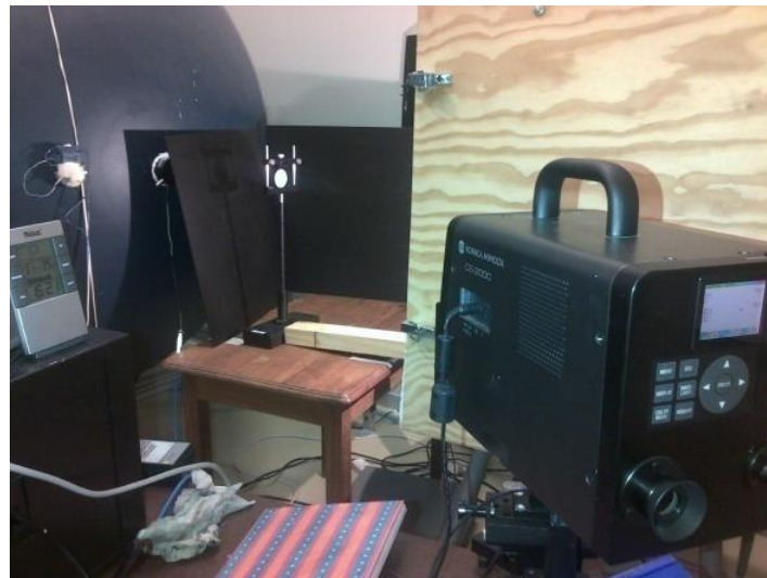
Figure 4.2. (a) A portable spectroradiometer used at UP
