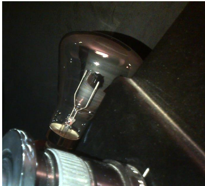
Figure 4.5. A tungsten filament illuminant A lamp from NMISA
