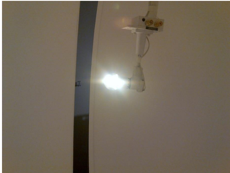
Figure 4.11. A 4000K CCT white LED lamp total luminous flux measurement
