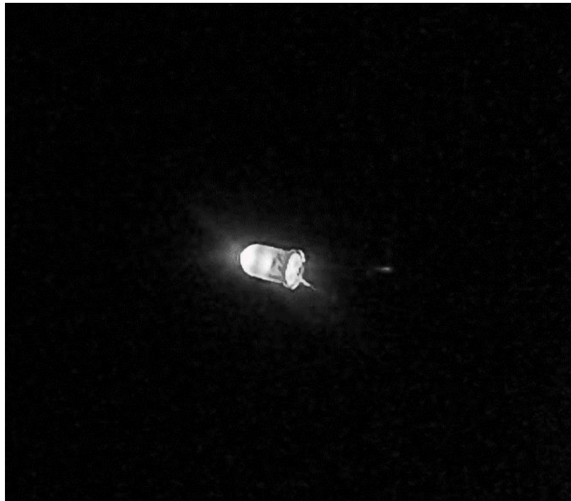
Figure A.4. A 5mm epoxy LED set-up for intensity measurement, showing its complex spatial distribution and back emissions
