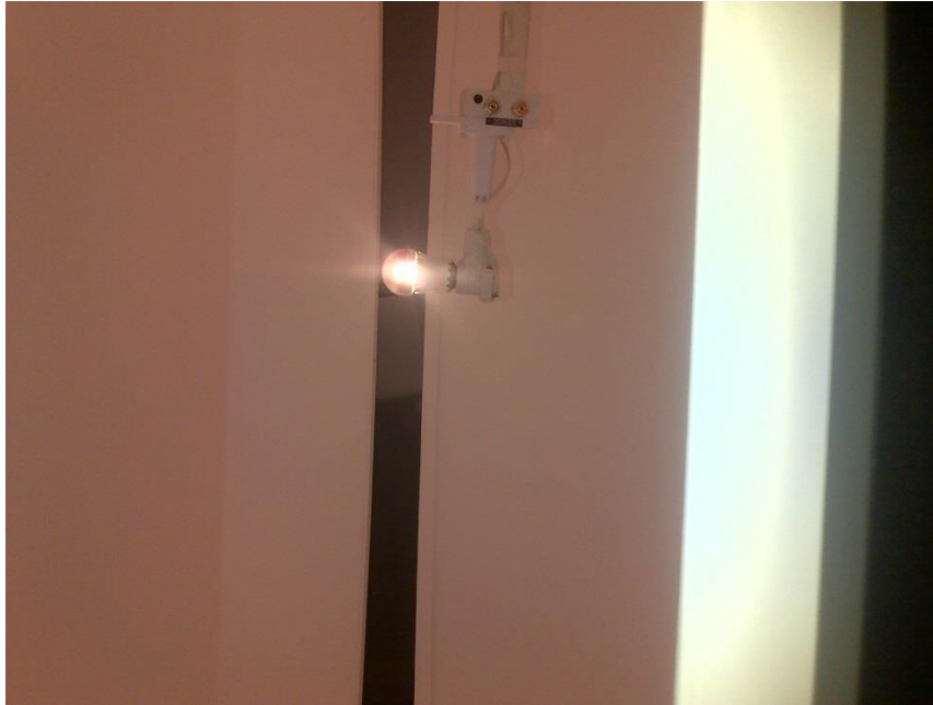
Figure A.12. A warm white Pharox LED lamp total luminous flux measurement using an integrating sphere
