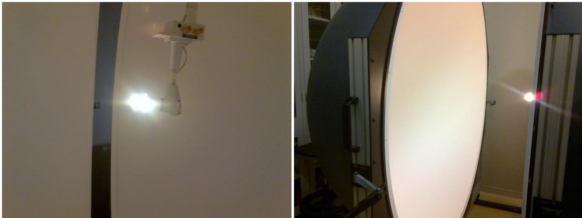
Figure 4.8. A Pharox 400 lm rated white LED lamp allowed to stabilise for 30 minutes inside an opened sphere before photo-diode measurement is taken
