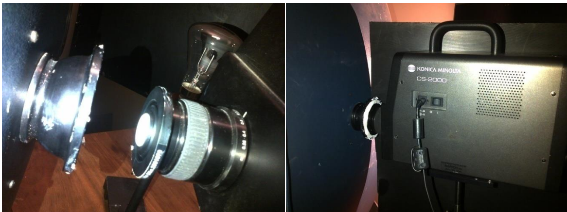
Figure 4.3. Measuring the relative spectral responsivity of the integrating sphere
