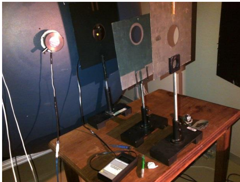
Figure 4.6. Set-up for calibration of the sphere sensitivity
