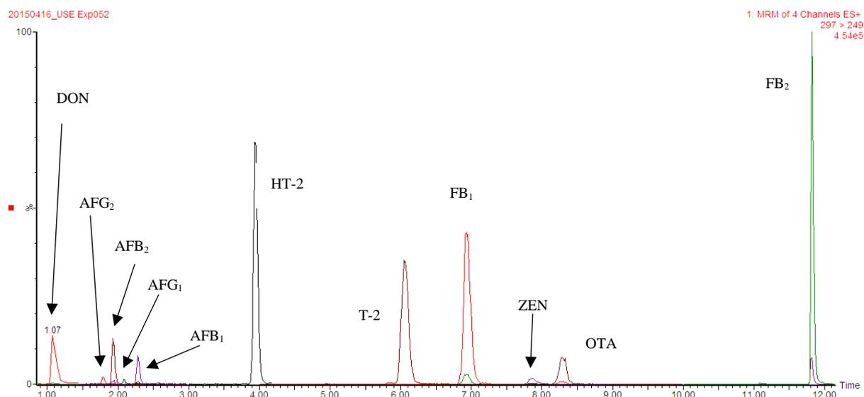
**Figure 4. 1.** Extracted ion chromatogram (XIC) of a blank maize spiked after extraction with labelled and unlabelled mycotoxins. Corresponding analyte spiking concentration and retention times are in Table 4.1.
