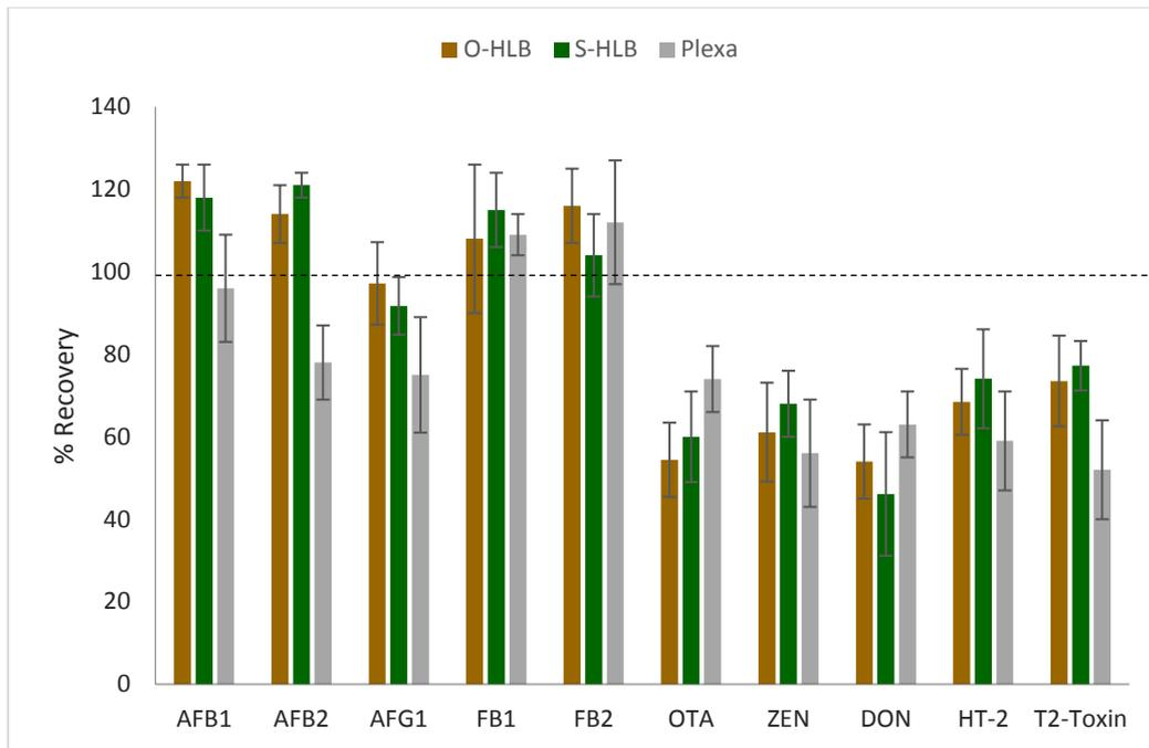
**Figure 4. 5.** Recoveries of naturally contaminated maize sample (Trilogy) ( $n = 3$ ); concentration levels given in Table 4.4.
