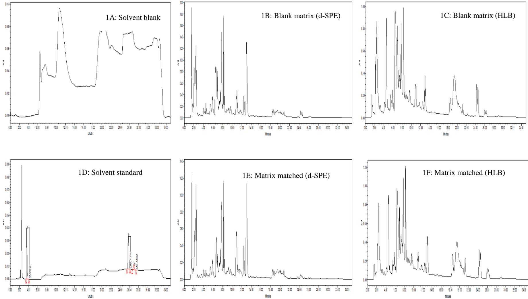
**Figure 4. 2.** Comparison of HPLC-PDA chromatograms for blank and spiked neat solvent and matrix matched calibration standards.
