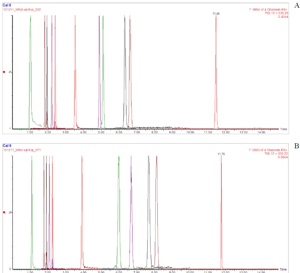
**Figure 4. 10.** Extracted ion chromatograms of solvent calibration standard obtained using Raptor ARC column (A) and Acquity BEH column (B). [<sup>12</sup>C]-AFB<sub>1</sub>, AFG<sub>1</sub>, 30 ng/g; AFB<sub>2</sub>, AFG<sub>2</sub>, 12 ng/g; FB<sub>1</sub>, 1500 ng/g; FB<sub>2</sub>, 750 ng/g; OTA, 75 ng/g; ZEN, 750 ng/g; DON, 1500 ng/g; HT-2 Toxin, T-2 Toxin, 1500 ng/g. Corresponding analyte and retention time are listed in Table 4.1.
