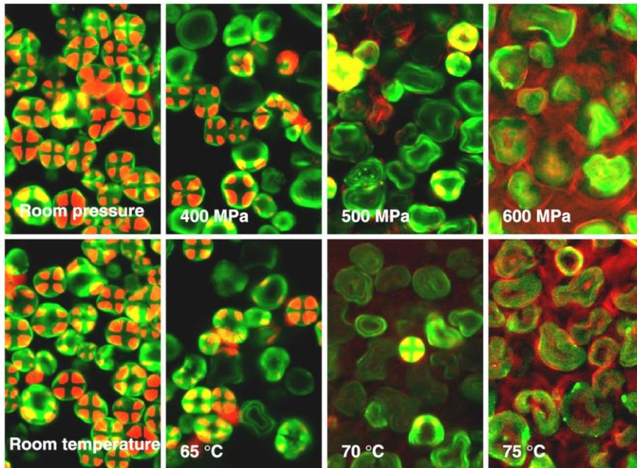
**Figure 2.11:** CLSM images of sorghum starch at different pressure and temperatures (Vallons and Arendt, 2009).
