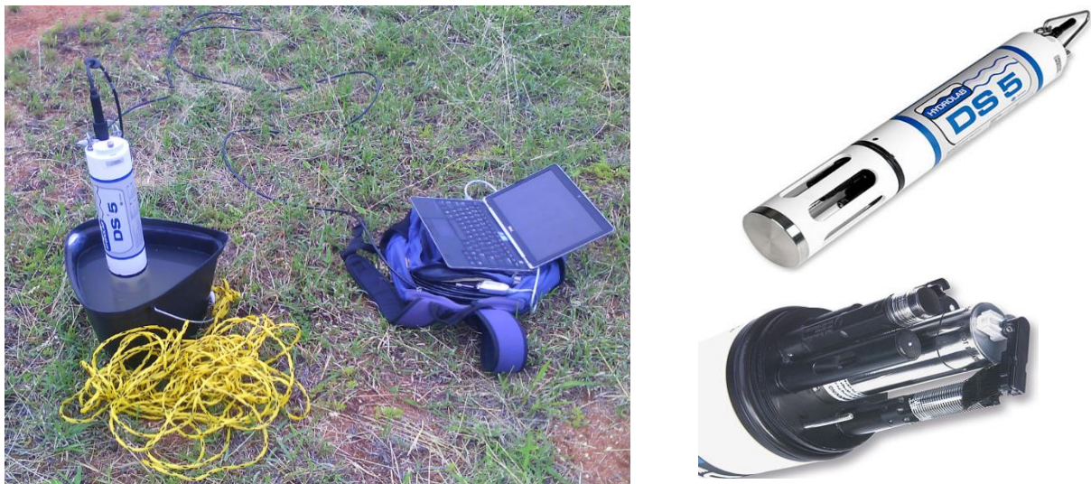
Figure 10: Experimental setup using Hydrolab DS 5 Multipleparameter Data Sonde
