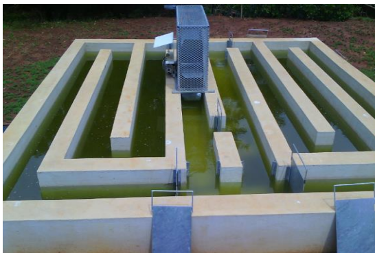
Rectangular shaped raceway pond with algae culture
