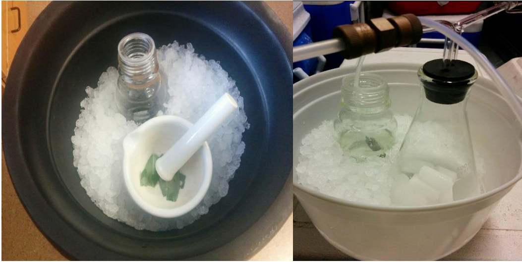
Figure 2.3 Thawed leaf samples were ground in buffer solution in preparation for the CA activity measurement assay (left image). The right image shows CO 2 -saturated water in preparation.
