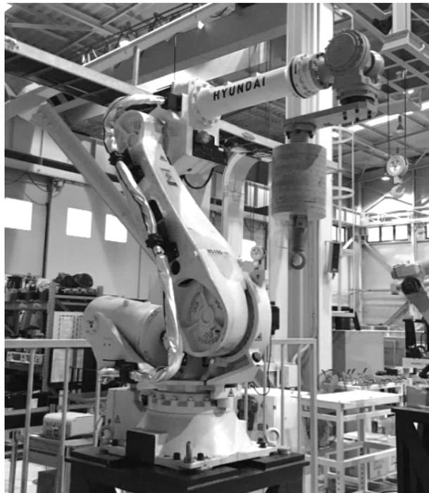
Figure 6.1. HS165 (Hyundai 6DOF industrial robot, maximum payload: 165 kg, main application: spot welding, <http://www.hyundai-robotics.com/robot/robot01.asp>).
