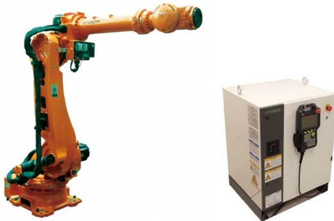
Figure 1.1. HS180 (left, 6 axis, payload: 180 kg, major application: spot welding and handling) and Hi5a controller and teach pendant (right, commercialized in 2008), used with permission of Hyundai Robotics Co., Ltd.
