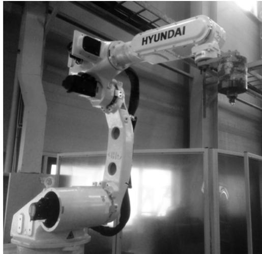
Figure 4.7. HA006B (DOF: 6, maximum payload: 6 kg, <http://www.hyundai-robotics.com/robot/robot01.asp>).
