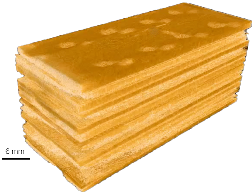
Figure 4.9 3D rendered volume structure of one half of the model spruce wood composites showing the wood veneer
