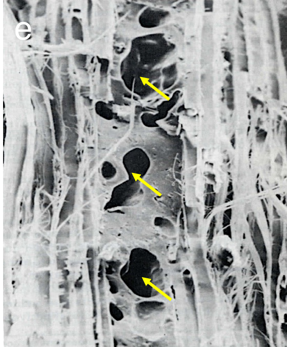
Figure 2.7 (a) Light microscopy; and (b ~ e) Scanning electron microscopy images of PF glue-lines in eastern spruce plywood: (a) Penetration of PF (dark areas) into ruptured cells; (b) Penetration of PF into a lathe check and close contact between adhesive and cell lumens; (c) Adhesive in resin canals and rays; (d) A uniformly thick glue-line; and (e) Voids in the glue-line (modified from figures in Hare and Kutscha 1974)
