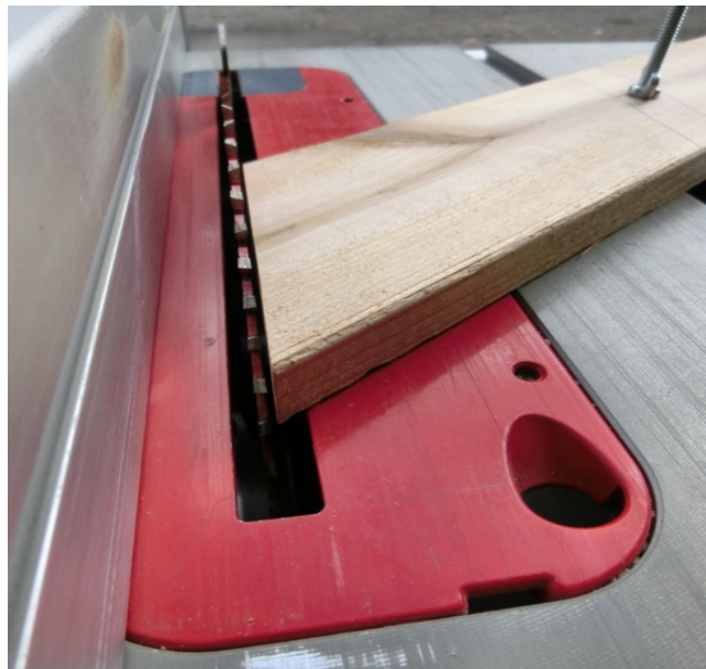
Figure 5.3 Table saw with a 25 cm (10") blade for cutting 1 mm thick veneers. The gap between the blade and the wooden guide which was clamped to the table of the saw was 1 mm
