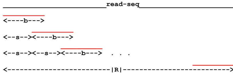
Figure 2.3: Querying the Bloom filter using a substring of length b .
