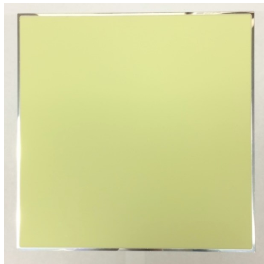
Figure 5.3: The flat-panel 193 mm \times 193 mm 1-mm-thick columnar CsI(Tl) scintillator.
