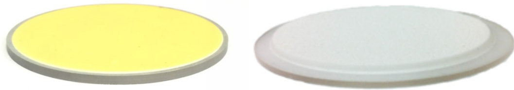
Figure 4.10: The original 450 \mu m columnar CsI(Tl) scintillator on FastSPECT III (Left) and the new 1.65mm columnar CsI(Tl) scintillator (Right).
