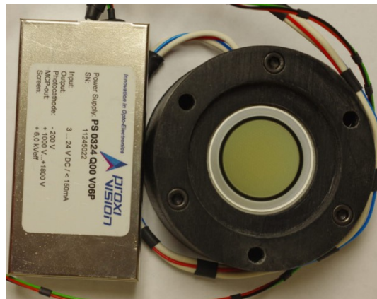
Figure 5.7: The 2-MCP image intensifier used in LA-iQID manufactured by ProxiVision in its 3D-printed custom housing.
