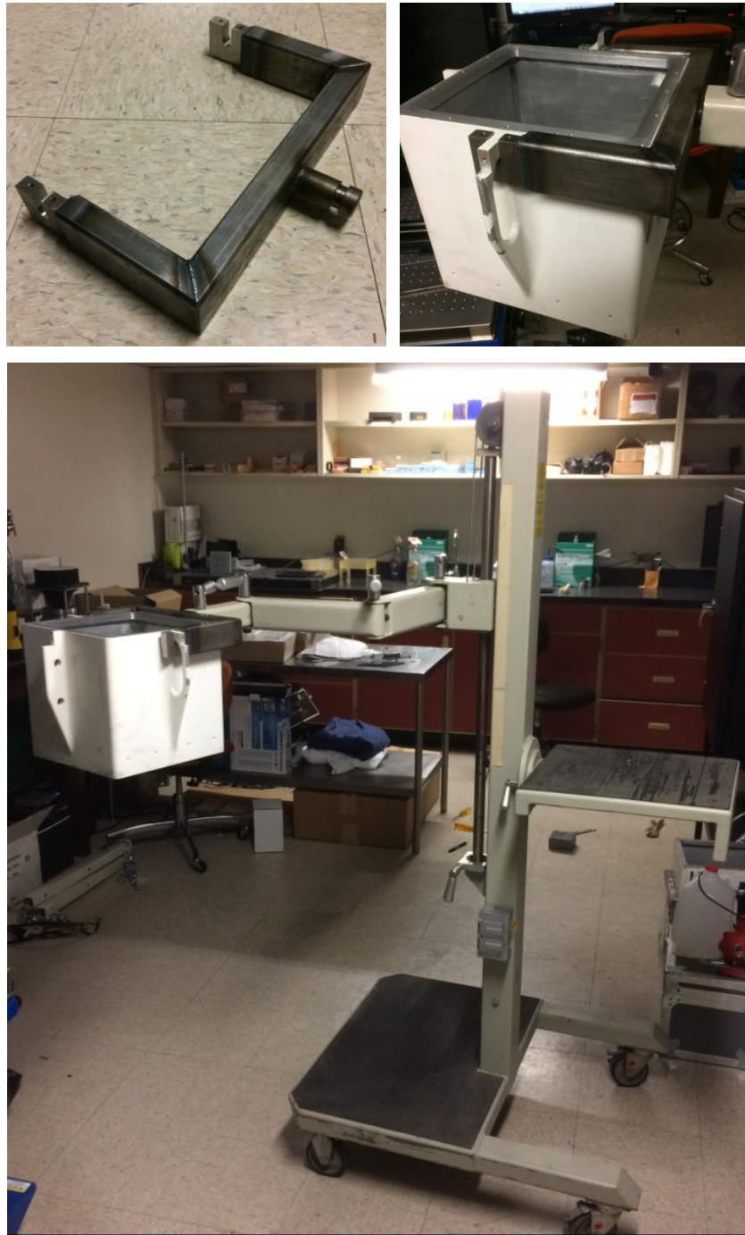
Figure 5.31: Top left: The customized steel holder with cylindrical pin for the LA-iQID camera. Top right: The external housing of LA-iQID held by the holder and attached to the arm of a clinical cart. Bottom: A photograph of the counter-weighted clinical cart with LA-iQID external housing attached through the custom holder.
