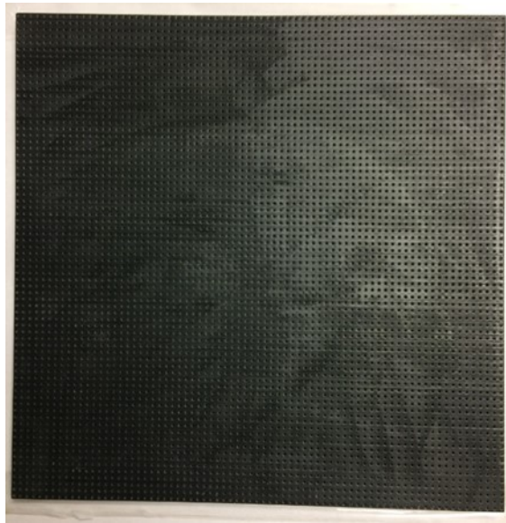
Figure 5.21: The 3D-printed calibration pattern with 74 \times 74 holes, 2.54-mm pitch and 5-mm thickness, each hole with 1-mm diameter.
