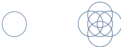
Figure 4.28: Projection images acquisition approaches. Left: 15-minutes acquisition with the phantom at the center of CFOV. Right: 15-minutes total acquisition with phantom at five different positions, each with 3-minutes acquisition.
