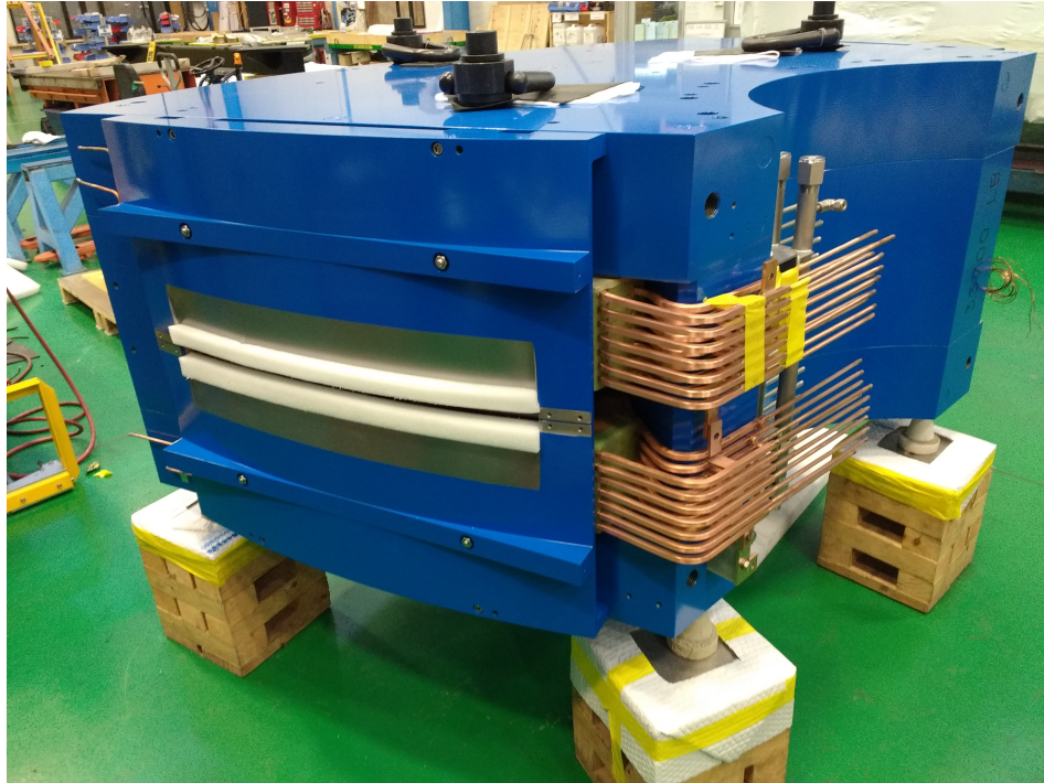
Figure 5.30: First HRS manufactured magnetic dipole (with field clamp edges protected by white Styrofoam). Photograph courtesy of Buckley Systems.
