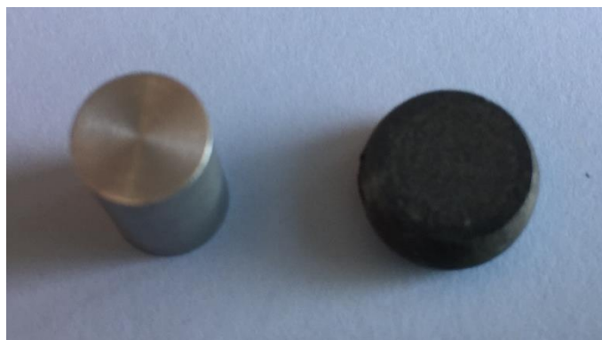
Figure 4-11 Pictures of samples taken before and after the high temperature compression test
