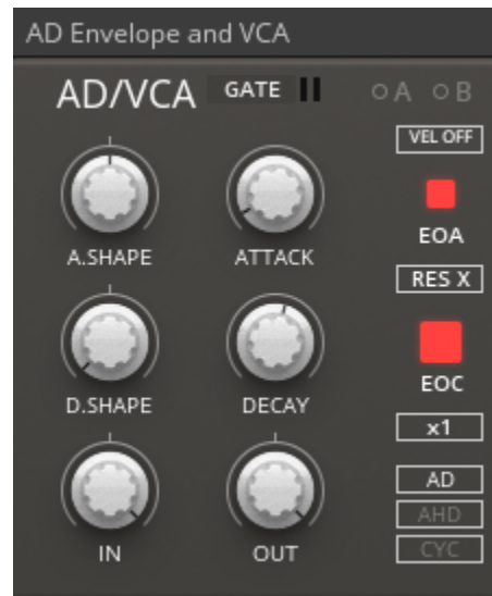
Figure 6.61: AD Envelope Panel
