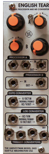
Figure 3.9: The Harvestman English Tear. This module acts as a translator between the 1 Volt Per Octave and Hz per Volt control voltage standards.
