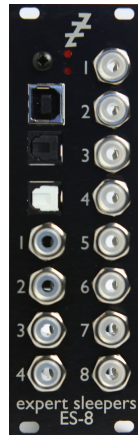
Figure 3.6: Expert Sleepers ES-8 USB Interface. Note the USB port in the top-left. This module provides DC-coupled inputs and outputs.
