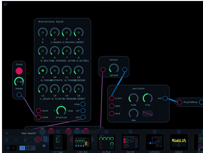
Figure 6.10: Audulus Modular. This screenshot shows both low-level “Nodes” like PolyToMono and higher level “Modules” like Bidirectional Seq16.
