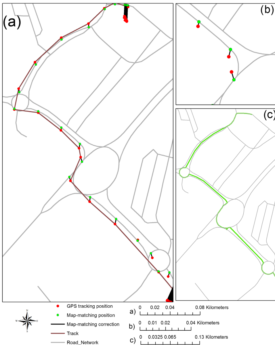
Figure 9. An example of map-matching an off-road track: (a) the off-road track, (b) the map-matching correction and (c) the trip after map-match.
