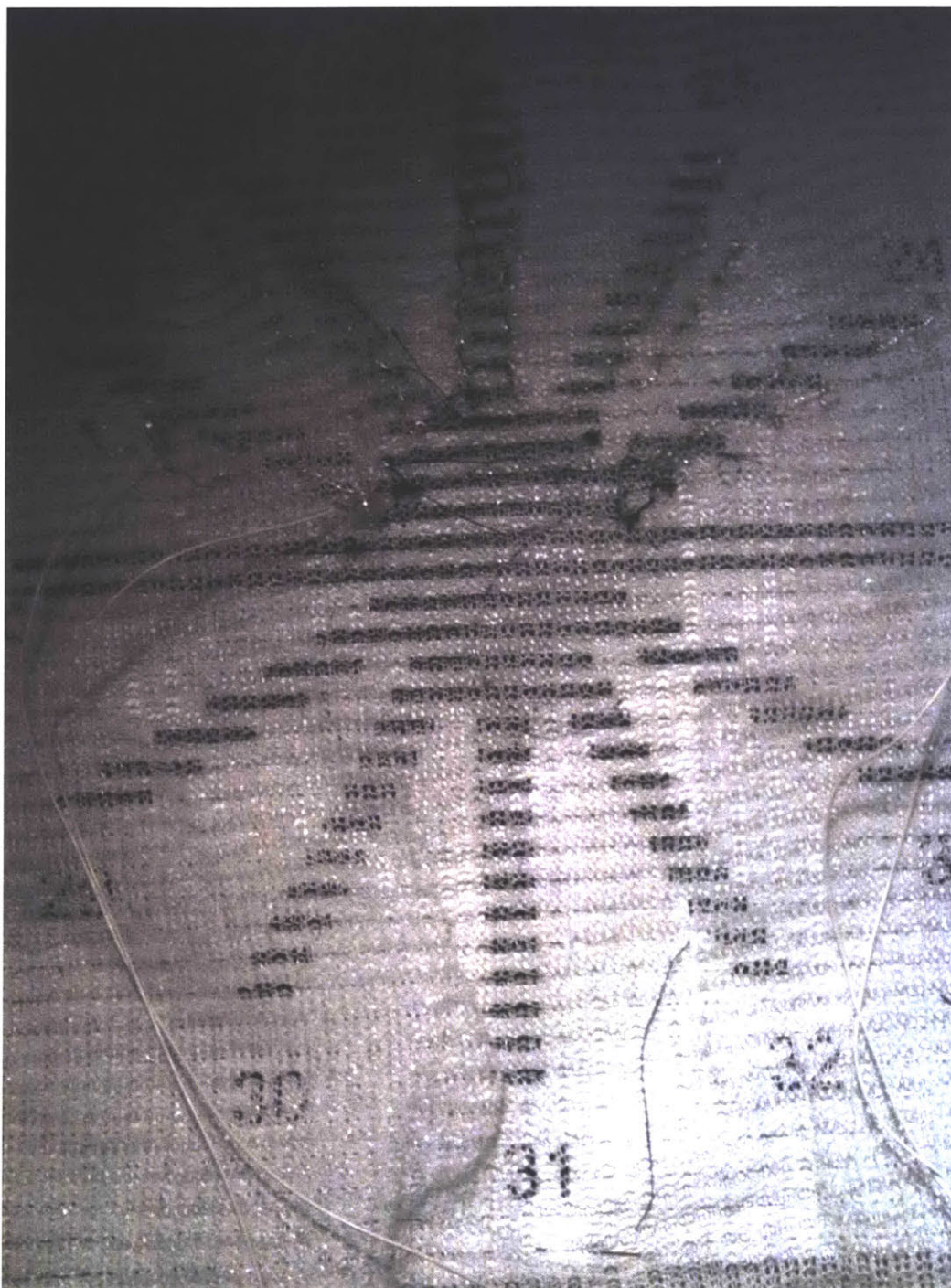
Figure 7.20. Sewing and cutting the circuits into the fabric on top of the Radiant Daisy Pattern.
