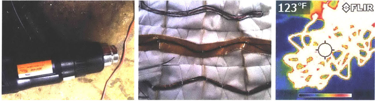
Figure 8.14. Heat gun and heat-shrunk plastic insulation for Nitinol wire (left), yellow high-temperature heat-resistant polyimide tape over Nitinol wire (middle), measured temperature of activated Nitinol wire (right).
