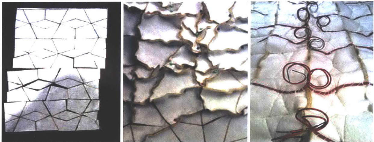
Figure 8.13. Laser-cut felt (left), pinned felt (middle), felt with sewn insulated Nitinol (right).
