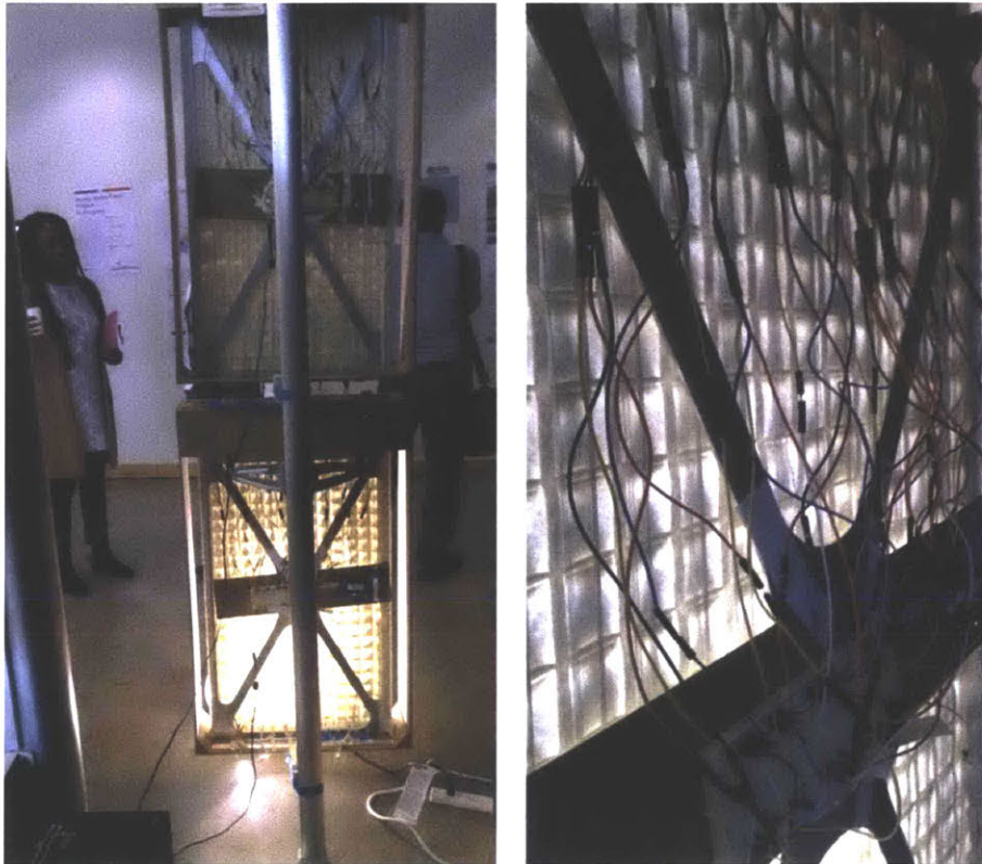
Figure 9.25. FELT: Preliminary mock-up back view (left); close-up of textile and wiring for servo motors (right).
