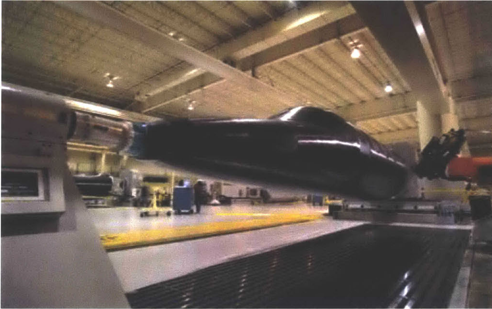
Figure 4.24. Beechcraft business jet fuselage, constructed using automated fibre placement. Photograph: Hawker Beechcraft (Sara Black, 2008). http://www.mmsonline.com/articles/getting-to-know-black-aluminum (Accessed 05-22-16).
