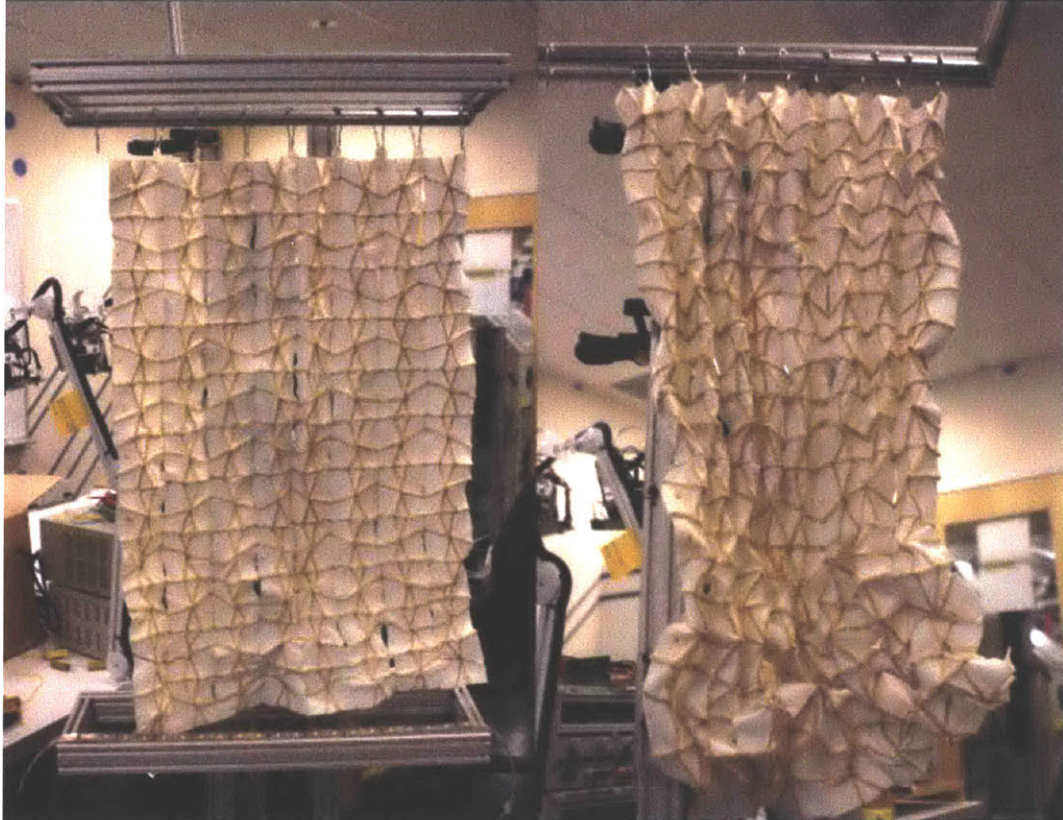
Figure 8.10. Canvas in a flattened state (left) and canvas in crumpled state (right).
