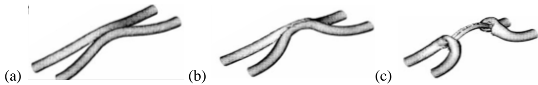
Figure 2.7: Three stages of vortex reconnection (a) induction, (b) bridging, (c) threading. Adapted from Marshall (2001).
